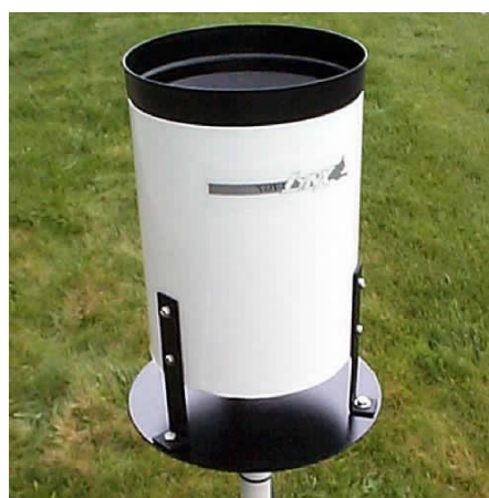
Figure 3. 16: Typical tipping bucket rain gauge
