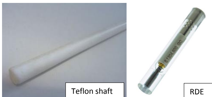
Figure 2.5: Pictures of the Teflon shaft and the RDE which can be used as stirrers.
