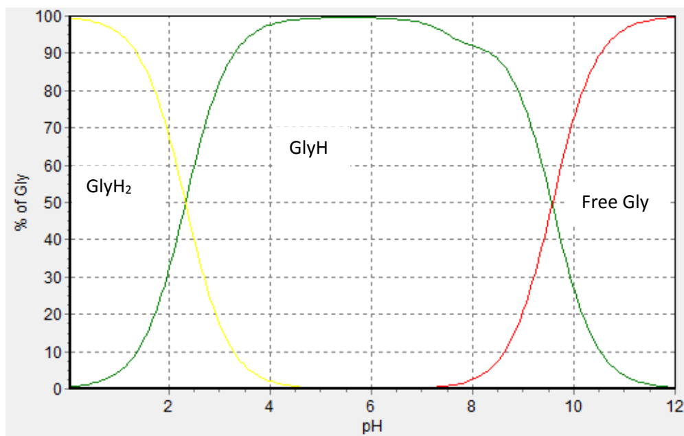
Figure A1.5: Species distribution diagram for the 0.1 M glycine in \text{HNO}_3 . The species distribution diagram was plotted using the protonation constants in Table A1.3 at 25°C and the indicated ionic strengths.
