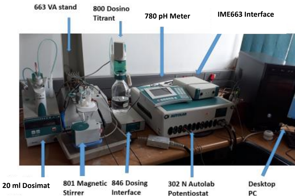
Figure 2.2: Metrohm Autolab Instrumental setup used for all voltammetric measurements.
