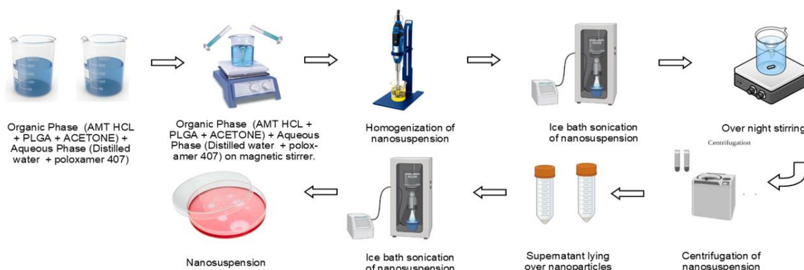
Figure 3.1 Schematic representation of preparation of AMT-PLGA nanosuspension using nanoprecipitation.
