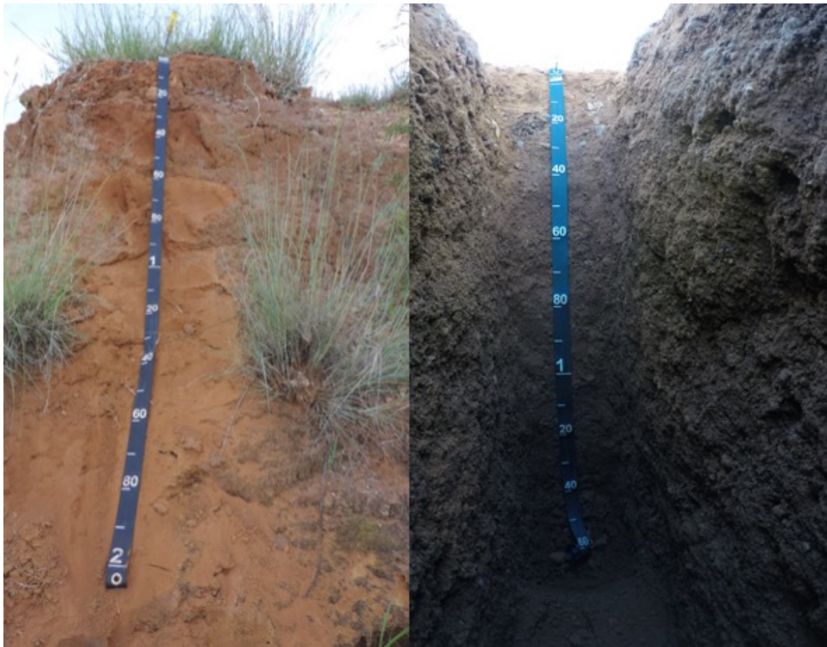
Figure 7: Photographic evidence of an undisturbed Hutton soil profile indicating red apedal soils of 2m deep without any impediments (left) and a rehabilitated mine soil profile high in rock fractions limited in depth at 1.6m because of compaction (right)
