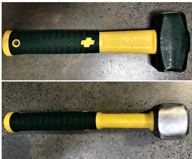
Figure 3.2. Steel mallet used to inflict BFT to adult-sized pigs. The weight of the mallet is 1.1 kg, with the head measuring 50 x 50 mm.
