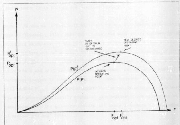
Figure 8. Relationship between P and F showing the desired operating point and a shift in this point due to a disturbance
