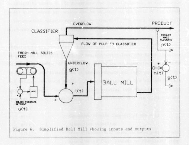
Control Objective: The control objective is to maximise the mill mass throughput given the constraint on size of product.
