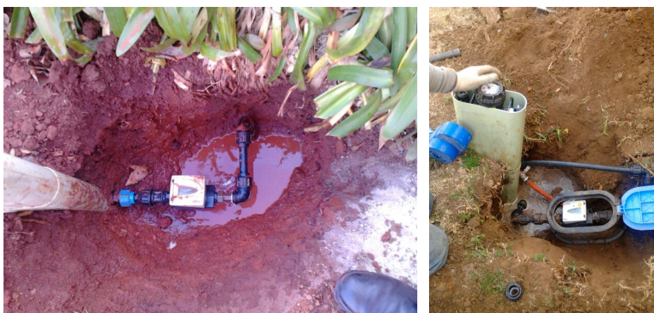
Figure 3-6: Meter Logging for Small Meters
