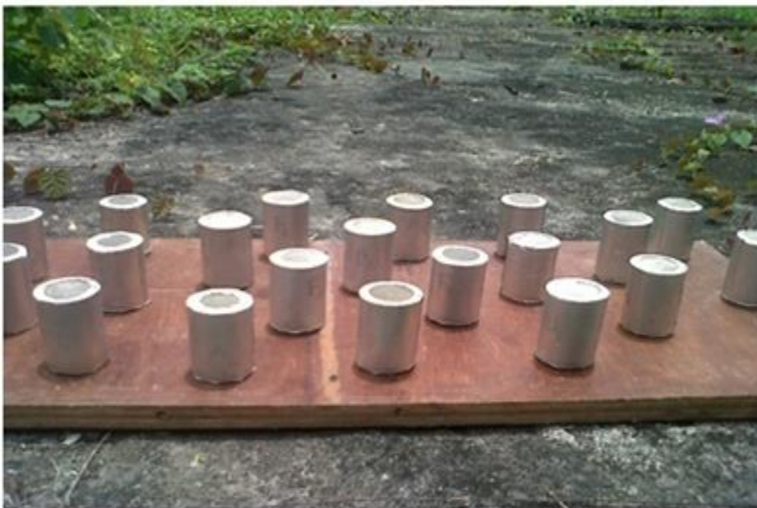
Figure 3.5: Agbada sandstone reservoir core plugs used in this work
