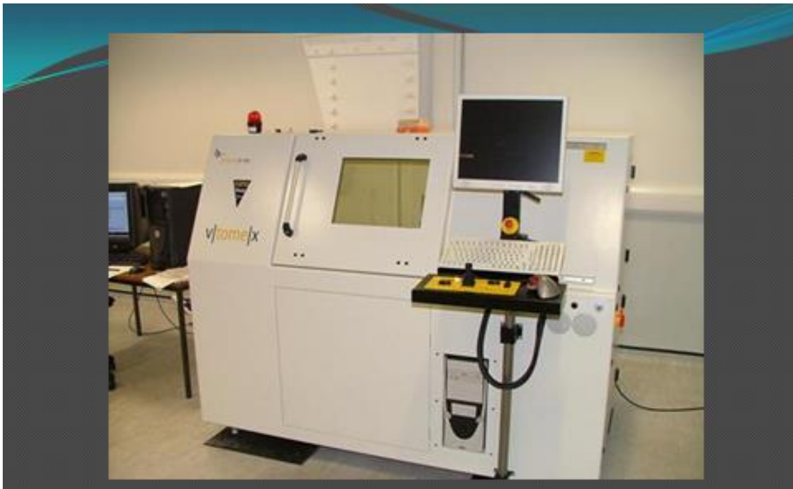
Figure 3.13: Micro-CT scanner, Phoenix vltomelx, at Imperial College, London
