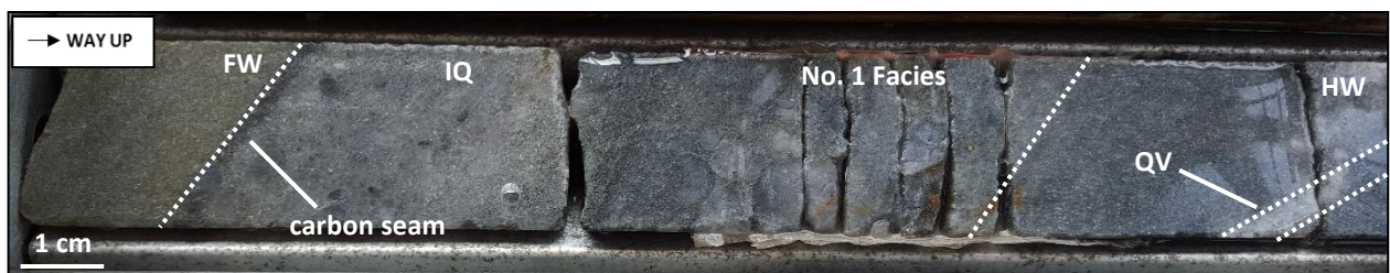
Figure 3.14: Matrix-supported No. 1 Facies with a siliceous internal quartzite (IQ) and an underlying carbon seam, separating the reef package from the footwall (FW) quartzite. A 5 mm thick quartz vein (QV) was seen cutting the hangingwall (HW) quartzite overlying the reef package – Sample 32.
