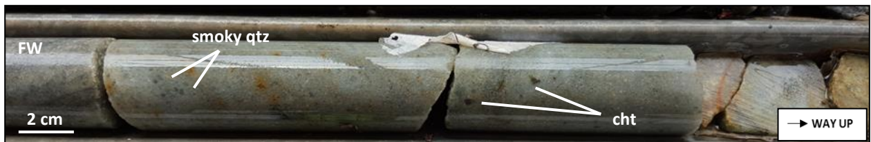
Figure 3.10: Greenish-grey argillaceous footwall (FW) quartzite with small floating clasts of rounded smoky quartz (qtz) and elongated to angular chert (cht) – Sample 23.
