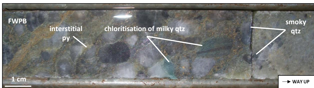
Figure 3.7: Footwall pebble band (FWPB) with possible chloritisation of some milky quartz (qtz) clasts. Smoky quartz clasts as well as interstitial pyrite (py) was also noted within the footwall pebble band – Sample 20.
