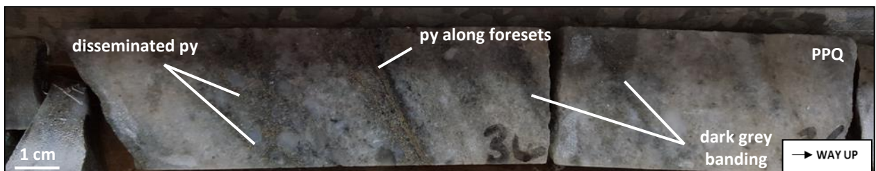
Figure 3.20: Pale Pebbly Quartzite (PPQ) intersection within the No. 2 Facies. The Pale Pebbly Quartzite had rounded disseminated grains of pyrite (py) as well as pyrite along foresets – Sample 35.
