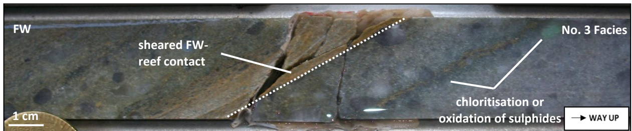
Figure 3.25: A close-up of the footwall (FW)-reef contact of the No. 3 Facies. Discolouration was noted on the edges of pyrite along foresets and may be due to oxidation of sulphides or chloritisation within the core – Sample 21.
