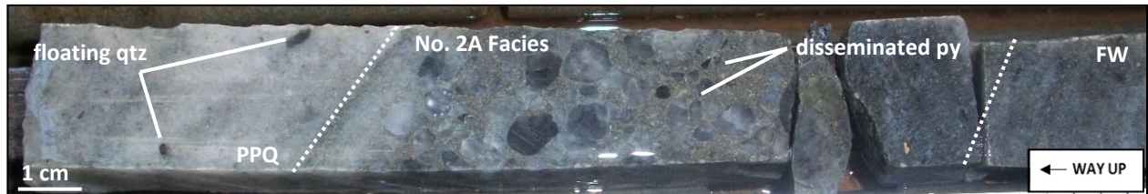
Figure 3.19: Matrix-supported No. 2A Facies with interstitial disseminated pyrite (py) between milky and smoky quartz (qtz) clasts. The No. 2A Facies was overlain by a Pale Pebbly Quartzite (PPQ) with floating quartz clasts – Sample 22.
