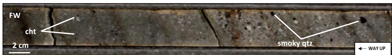
Figure 3.12: Floating chert (cht), smoky and milky quartz (qtz) clasts scattered across a gritty-textured footwall (FW) quartzite – Sample 48.
