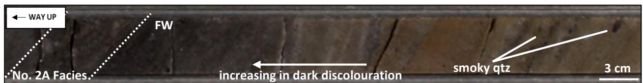
Figure 3.11: Discolouration (darkening) of the footwall (FW) quartzite closer to the No. 2A Facies. Floating clasts of smoky quartz (qtz) are also noted within the footwall quartzite – Sample 44.
