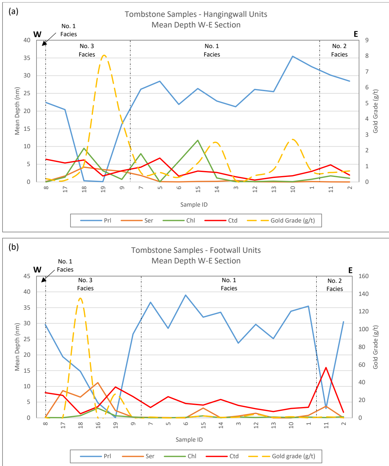
Figure 3.63: (a) Spectral mean depths (nm) of pyrophyllite (Prl), sericite (Ser), chlorite (Chl) and chloritoid (Ctd) of the hangingwall units overlying the Carbon Leader Reef in west-east section across TauTona Mine, plotted against gold grade (g/t); (b) Spectral mean depths (nm) of pyrophyllite (Prl), sericite (Ser), chlorite (Chl) and chloritoid (Ctd) of the footwall units underlying the Carbon Leader Reef in west-east section across TauTona Mine, plotted against gold grade (g/t).
