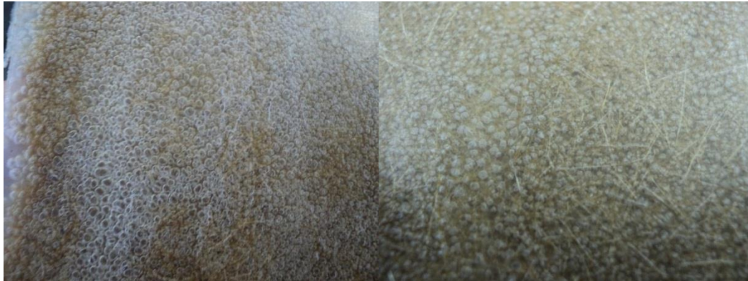
Fig. 122 Bubbles formed inside the composite
