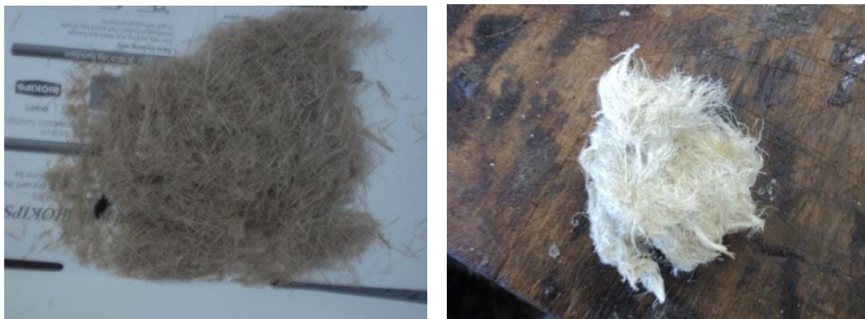
Fig. 34 Left: untreated fibres \ Right: treated fibre
