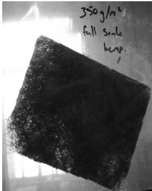
Fig. 20 Hemp fibre mat at a density of 350 g/m 2
