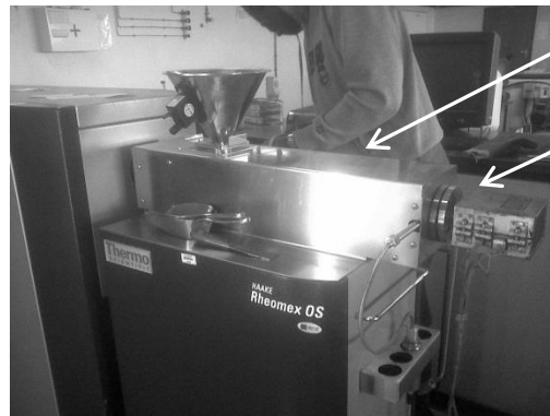
Fig. 22 Haake Polylab with extruding die used in the present work
