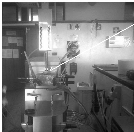
Fig. 23 Haake Polylab with shear mixer attached used in the present work
