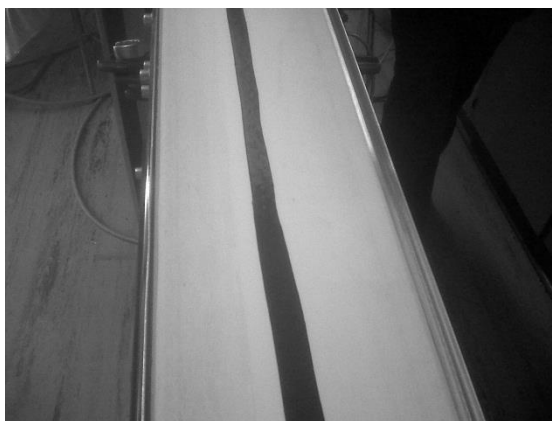
Fig. 35 Extruded polypropylene and carbon nanotube sheets
