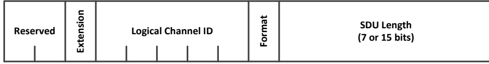
Figure 4.6: The 3GPP LTE MAC PDU Header Format for DL-SCH and UL-SCH [17, 19, 30–32, 38, 107]
