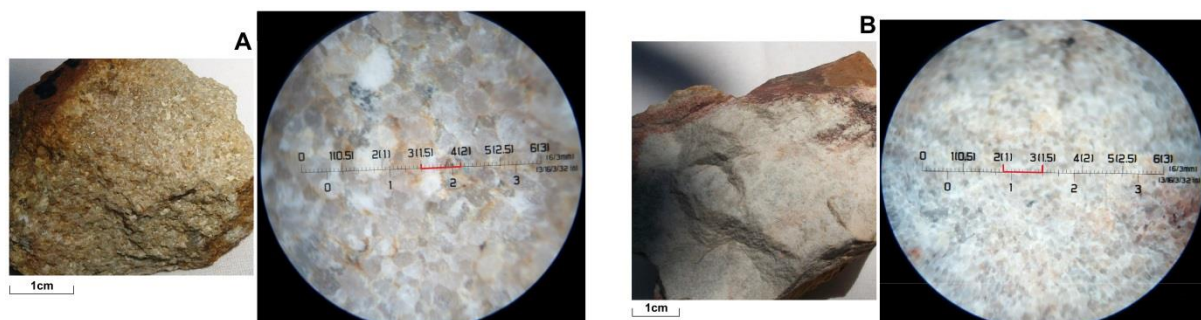
Fig. 6. Grain size visible using the Macroscope M25, the red line is 1mm (Adapted from Sherwood {2013}).
