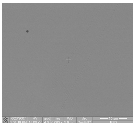
Figure 4.138. BEI of LG 11 (Nominal Co 40 :Pt 50 :Ru 10 ) after ordering heat treatment and water quench consisting of the CoPt phase.
