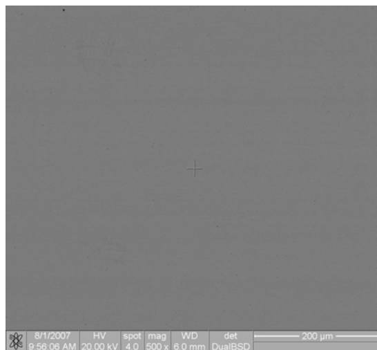
Figure 4.141. BEI of LG 12 (Nominal Co 15 :Pt 75 :Ru 10 ) after ordering heat treatment and water quench consisting of single phase (Pt) .
