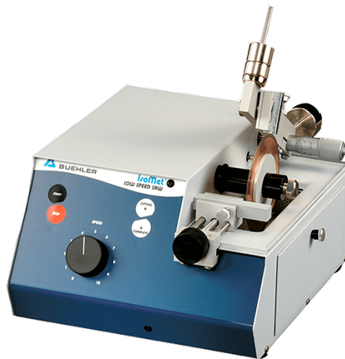
Figure 3.9: Buehler IsoMet LS [51]
