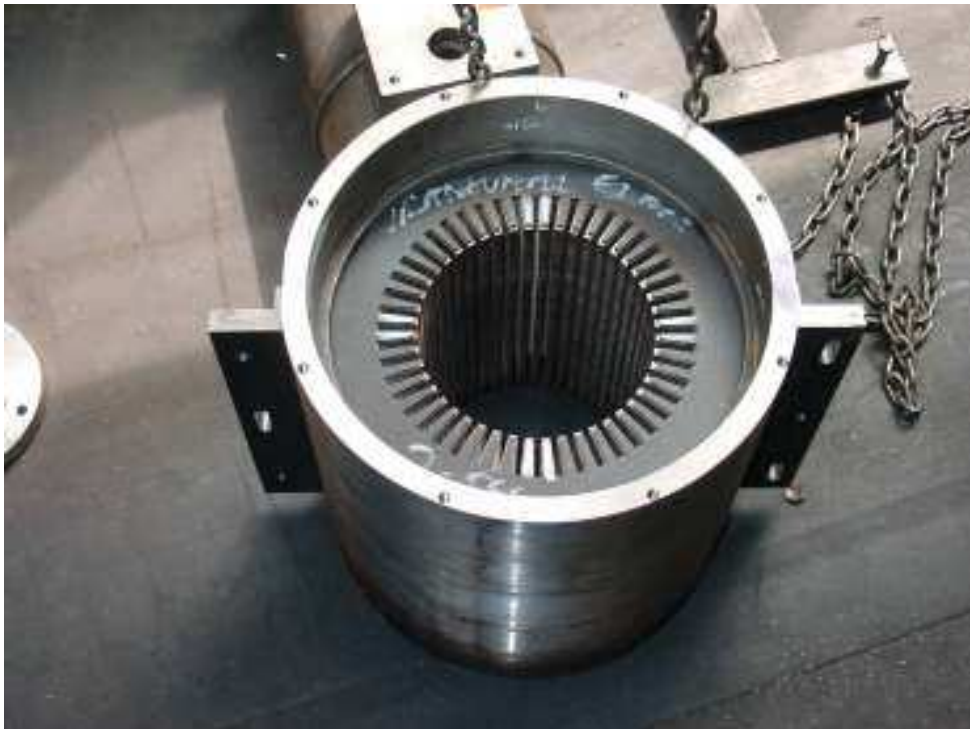
Figure 3.8: Photo of the stator during construction with casing
