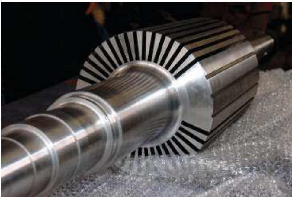
Figure 3.6: Photo of the rotor during construction with empty slots
