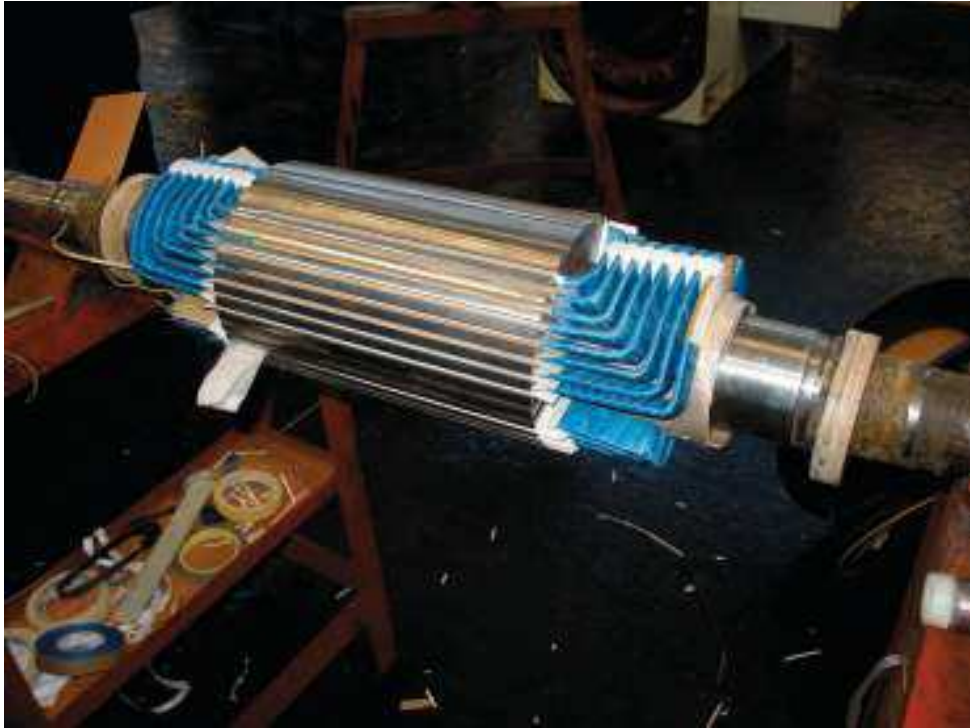
Figure 3.7: Photo of the rotor during construction with field winding
