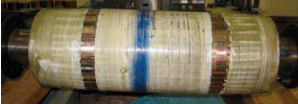
Figure 2.6: The rotor with sections of resi-glass removed near the ends of the core to allow for a direct air gap measurement
