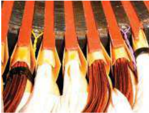
Figure 2.10: Two search coils in the grooves of the stator teeth with twisted leads
