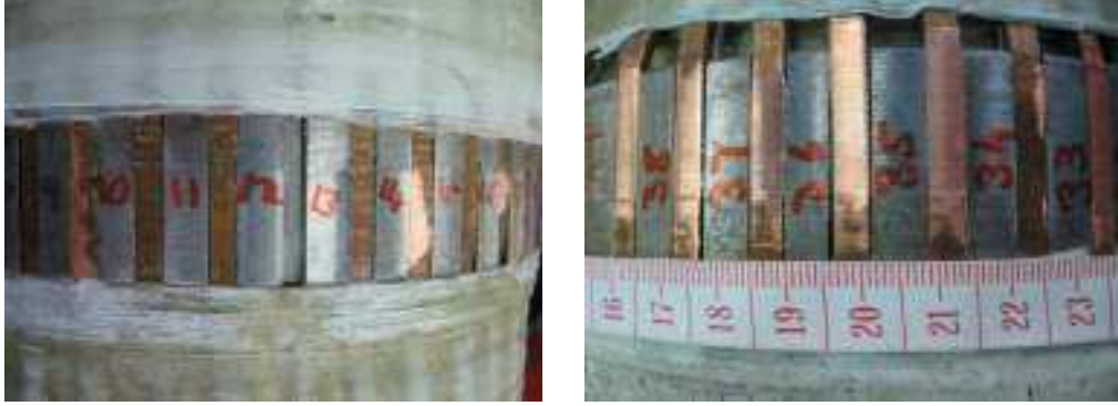
Figure 5.10: Upon removal of part of the resi-glass covering on the rotor, a slot without a damper bar and various other slot distortions were discovered
