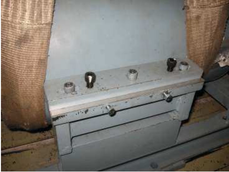
Figure 2.7: Bolts in the stator supports are used to adjust the alignment of the stator relative to the rotor
