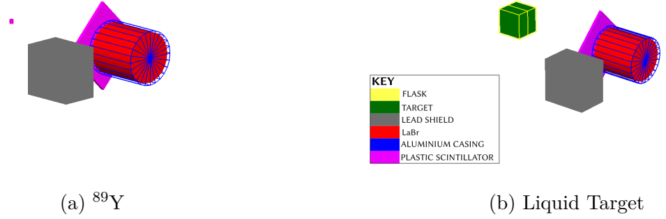
Figure 2.7: TOPAS Simulation Setup. Common geometries found in both solid and liquid target set-ups: scintillator (seen as the magenta 45^\circ box), LaBr_3:Ce detector with its aluminium casing (seen as red cylinder), lead shield (seen as grey box).
