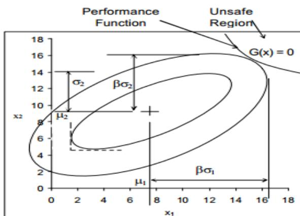
**Figure 2-14 Mean Points and Reliability Index in a Plane, after Myers et al. (2009)**
