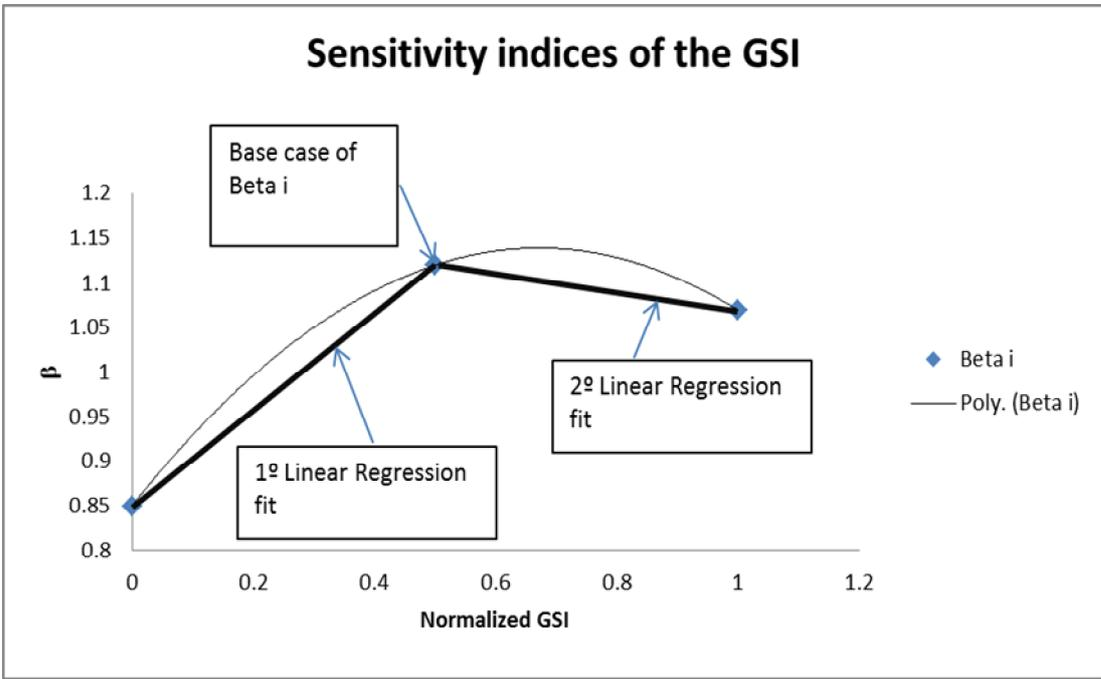
**Figure 4-1 Conversion of RSM polynomial curve into two regression lines**
