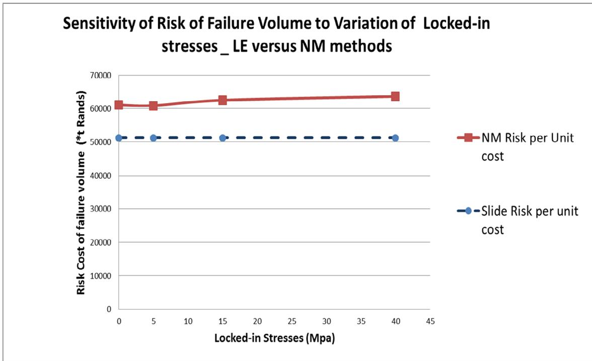
**Figure 5-32 Comparison of LE and NM risks of failure volumes to variation of LIS**
