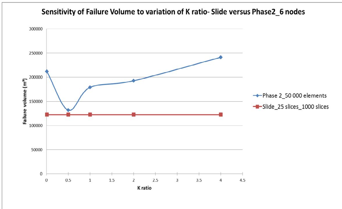
**Figure 5-27 Comparison of LE and NM failure volume sensitivities to variation of K ratio**
