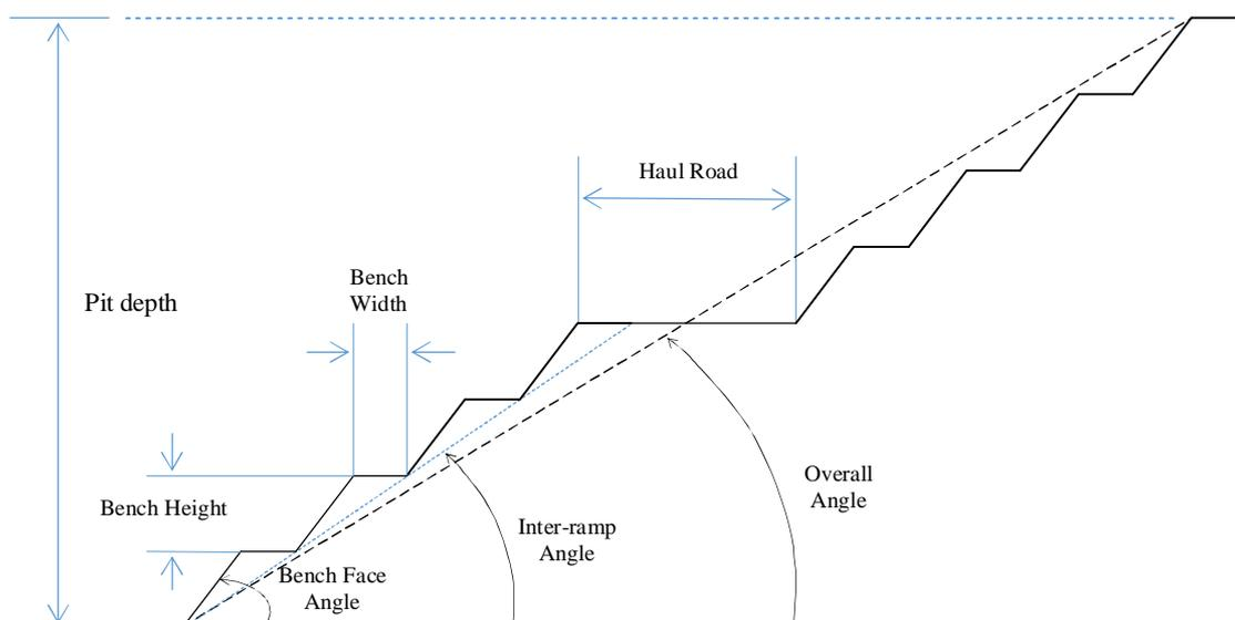
**Figure 2-1 Typical open pit design, after Hustrulid *et al.*, eds. (2000)**
