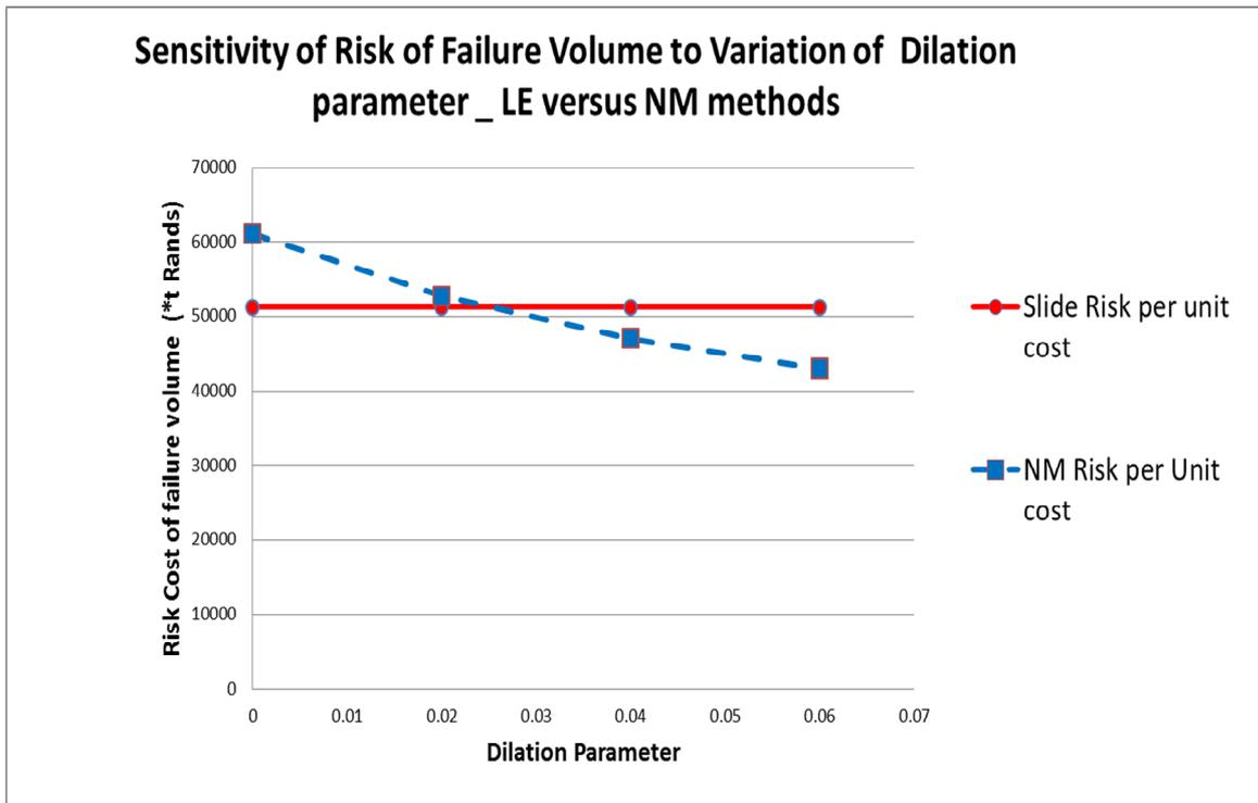
**Figure 5-36 Comparison of LE and NM risks of failure volumes to variation of Dilation parameter**
