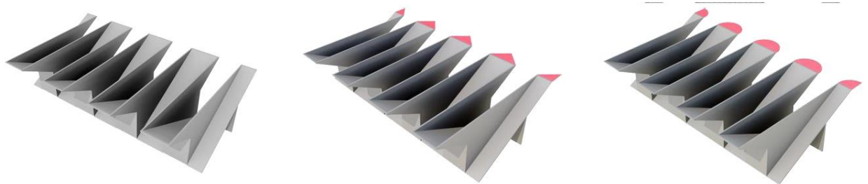
Figure 2.15: Sketches of Laboratory-scale PKW model (Left:Regular PKW; Middle: Triangular expansion at downstream of PKW; Right: Semi-circle expansion at downstream end of PKW), flow direction left to right (Oertel, 2015)
