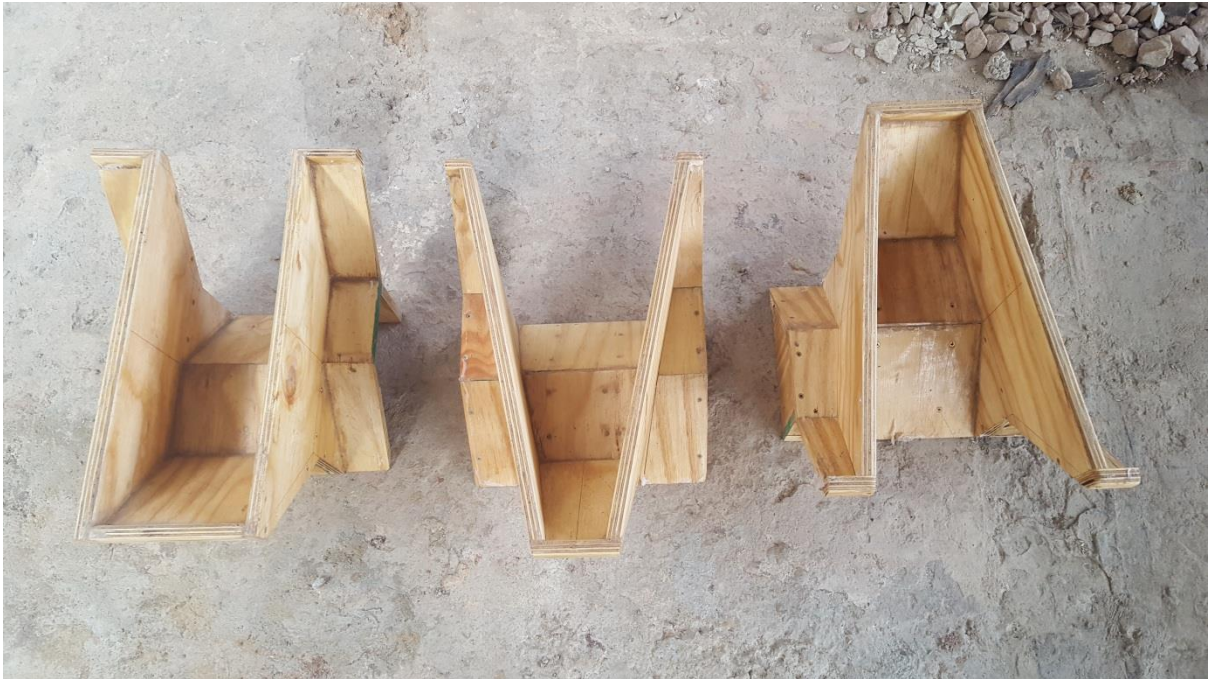
Figure 12.4: Models B3, B7 and B10 with the adjusted design consisting of a combined horizontal and sloping floor
