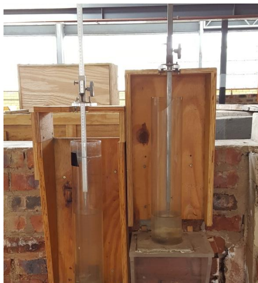
Figure 4.1: Stilling wells installed just next to flume to measure water surface elevations in flume
