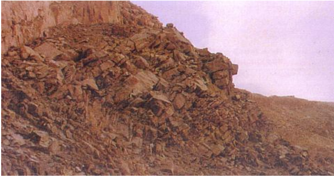
Figure 2.13: Bench-scale block toppling on joints in ganodiorite (After Lorig, et al. 2009).
