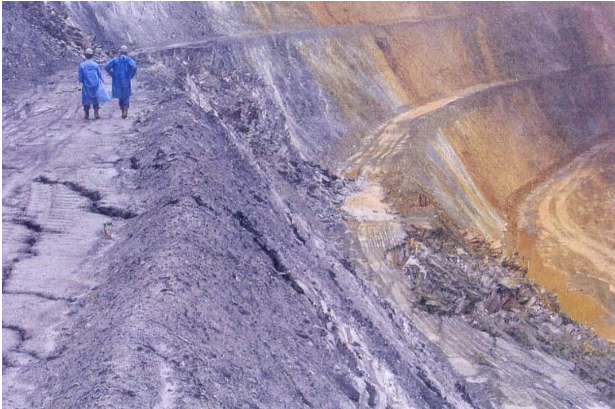
Figure 2.15: Bench-scale flexural toppling on cleavage in sericitic phyllite (After Lorig, et al. 2009).
