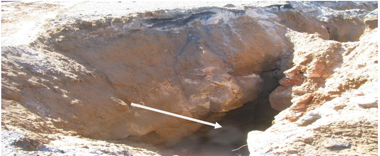
Figure 1.1: Sinkhole resulting from old underground workings at Kleinkopje open-cast coal mine.
