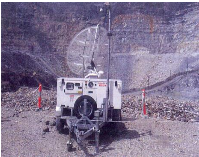
Figure 3.6: Slope Stability Radar (After Hawley, et al. 2009).
