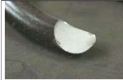
Figure 9.1.1: Fatigue failure on SCV54/03 at 162199 cycles
