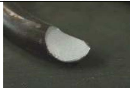
Figure 9.1.4: Fatigue failure on SCV54/03 at 897710 cycles.
