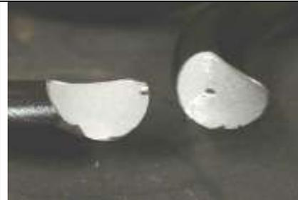
Figure 9.1.2: Fatigue failure on SCV54/03 at 298023 cycles.
