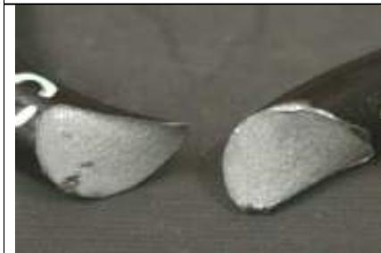
Figure 9.1.3: Fatigue failure on SCV54/03 at 421284 cycles.
