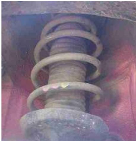
Figure 2.14.2: Application of coil spring in a suspension system.
