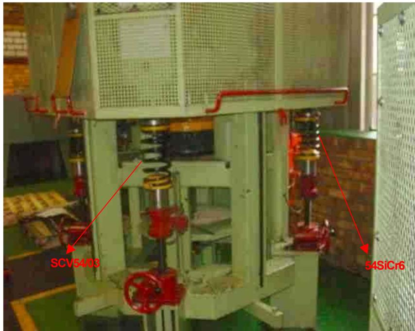
Figure 4.7.1: Test layout on fatigue testing machine.
