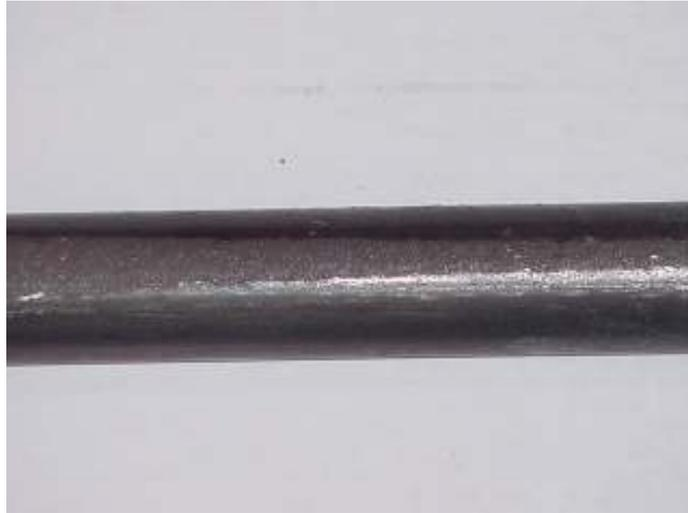
Figure 2.14.4: Bar in as rolled condition.
