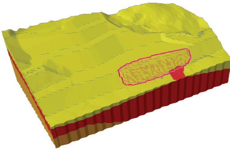
Figure 5: Initial 3D limit equilibrium stability analysis indicating an SF of 1.49 (McQuillan et al., 2020).
