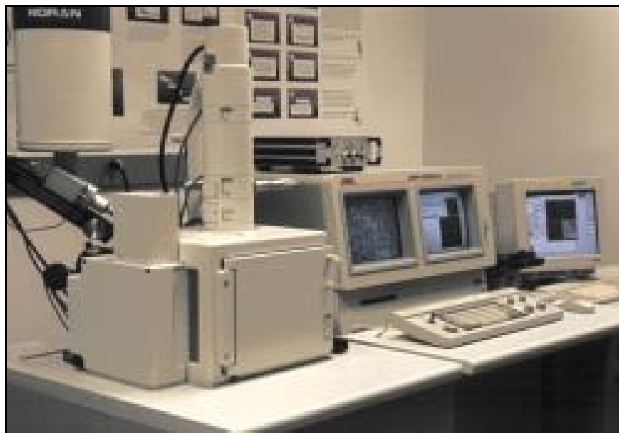
Figure 2.12: SEM instrument showing the electron column, sample chamber, EDS detector, electronics consoles and visual display monitors.
