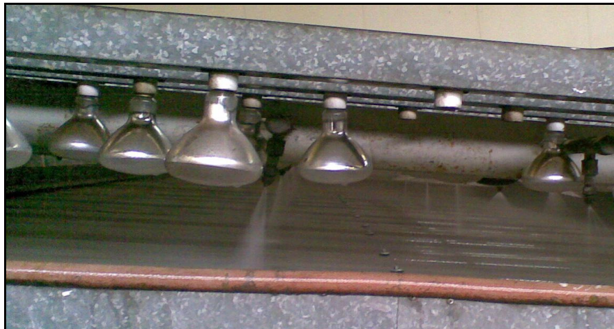
Figure 2.9 Rain cycles, simulating rainfall, evaluating permeability of sheets
