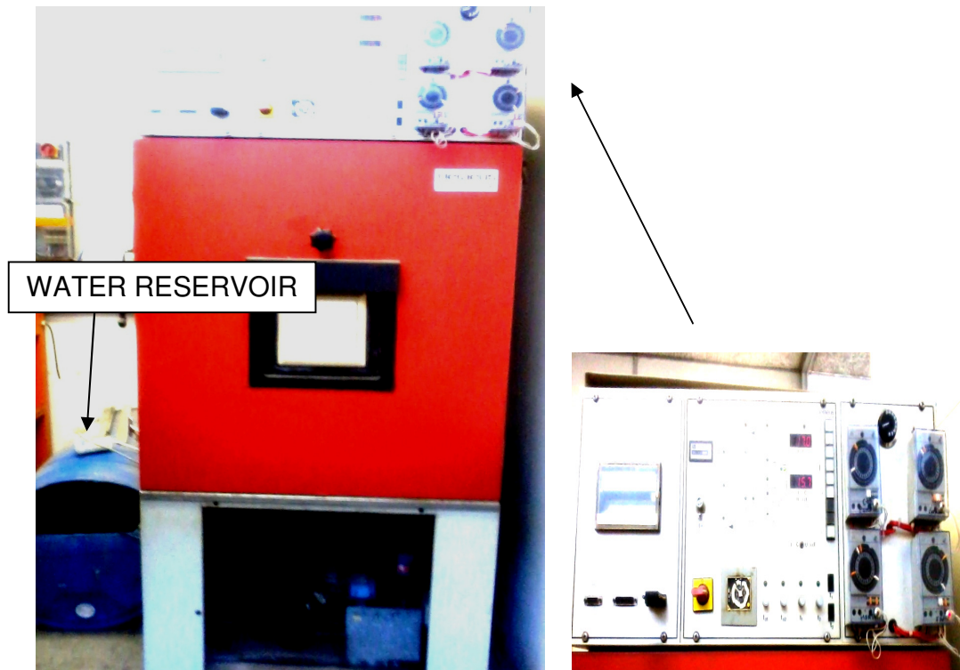
Figure 2.7: Accelerated carbonation chamber, with switches to change over from carbonation to ventilated oven to filling water bath with saturated water
