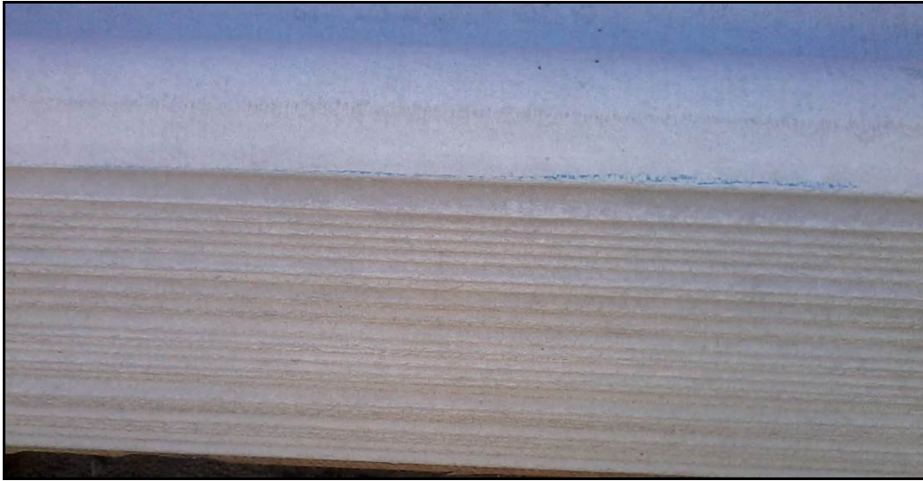
Figure 6.43: Corrugated sheets, 3% kaolin as replacement of cement, cured indoors without plastic wrapping. No cracks observed.
