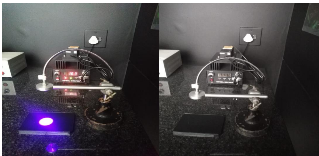
Figure 3.2 Laboratory images of the 405nm blue light diode laser (provided by CSIR) used in PDT studies.
