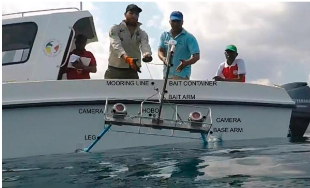
Figure 2. 4: Photograph of the stereo-BRUVS used to sample the sites in 2018 with annotations (from van Wyk, 2019)
