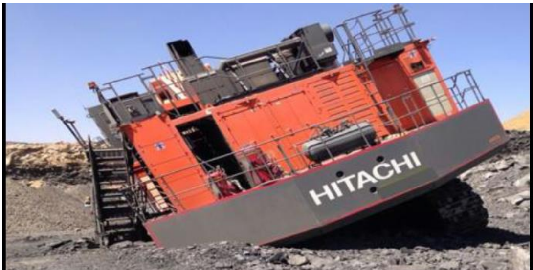
Figure 2-7: Face shovel falling into a void (Govender, 2018)
