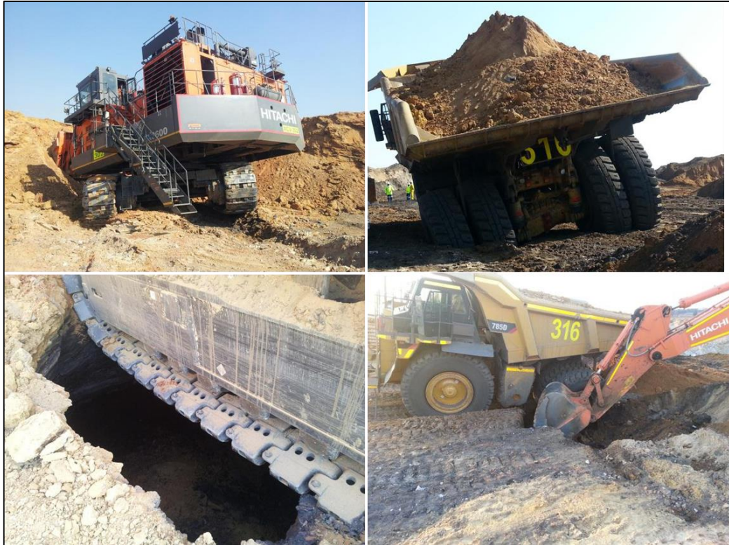
Figure 2-29: Face shovel and truck incident due to method 2 (Tweefontein Colliery, 2013).
