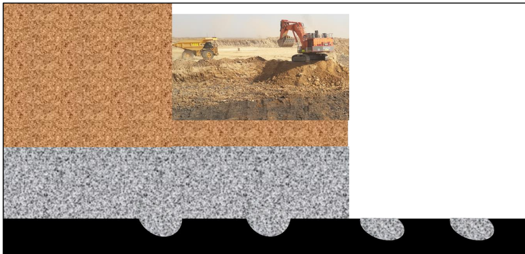
Figure 2-32: Coal profile after loading out waste material (Tweefontein Colliery, 2013)
