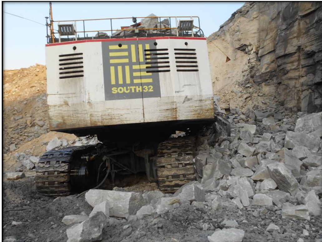
Figure 4-9: Highwall material fell on the shovel.
