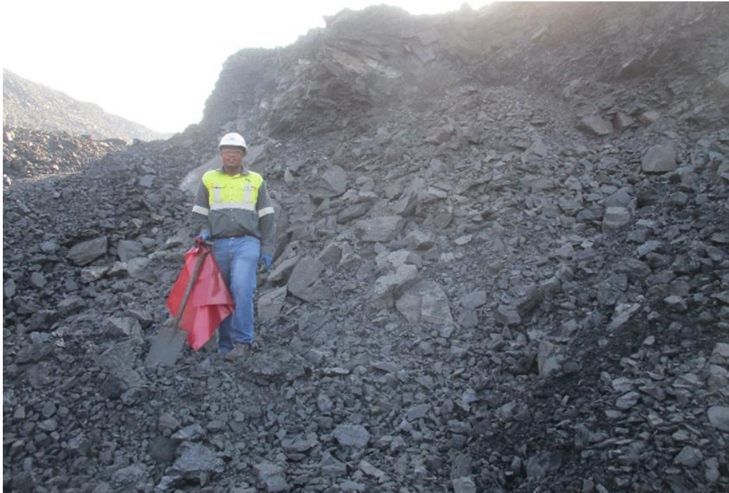
Figure 2-23: Collapsed coal pillar with shale contamination
