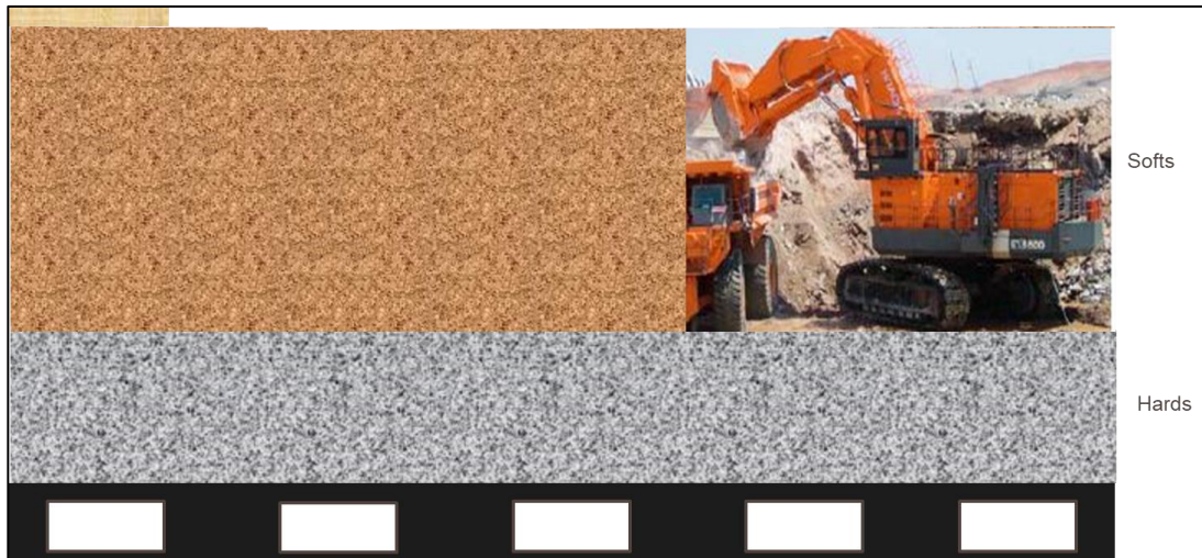
Figure 2-25: Face shovel prestripping soft material up to hard burden (Tweefontein Colliery, 2013)
