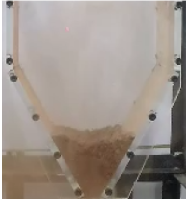
Figure 4.25: Profile of physical silo one eighth full of dry iron ore
