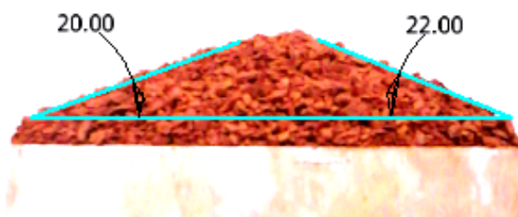
Figure K.3: Split pipe angle of repose, dry, physical test 3
