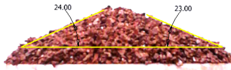
Figure M.3: Split pipe angle of repose, moist, physical test 3
