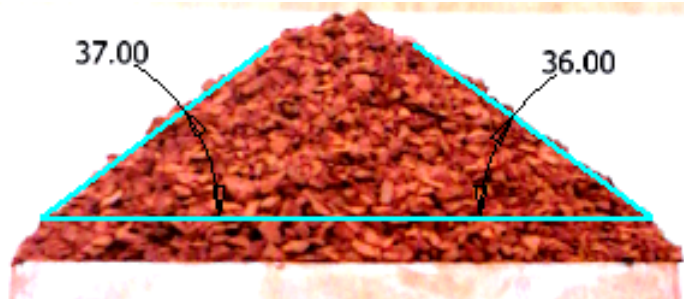
Figure J.5: Full pipe angle of repose, dry, physical test 2 @ 110 mm
