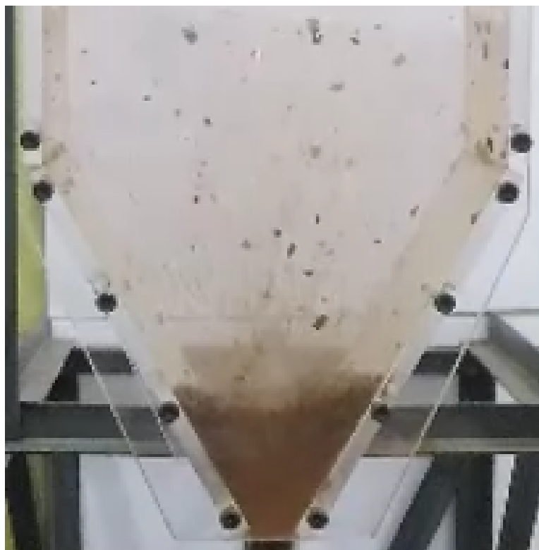
Figure 4.30: Profile of physical silo one eighth full of moist iron ore
