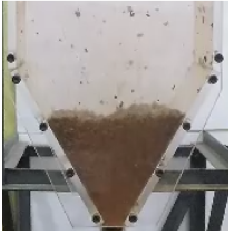
Figure 4.29: Profile of physical silo one quarter full of moist iron ore
