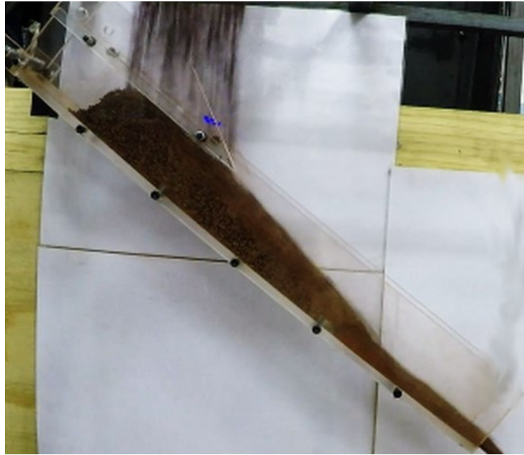
Figure 4.33: Profile of physical moist iron ore, chute steady flow
