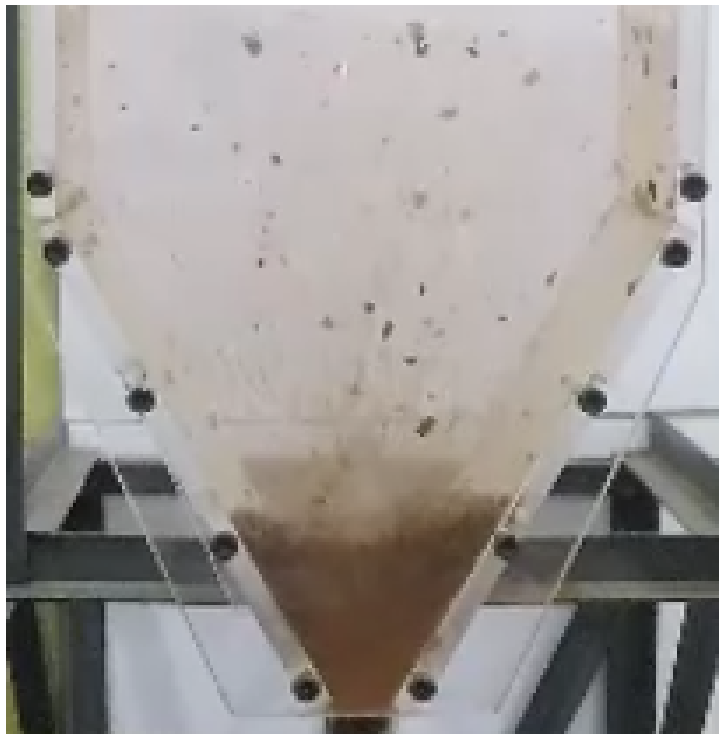
Figure 4.48: Flow profiles comparison, one eighth full silo, moist
