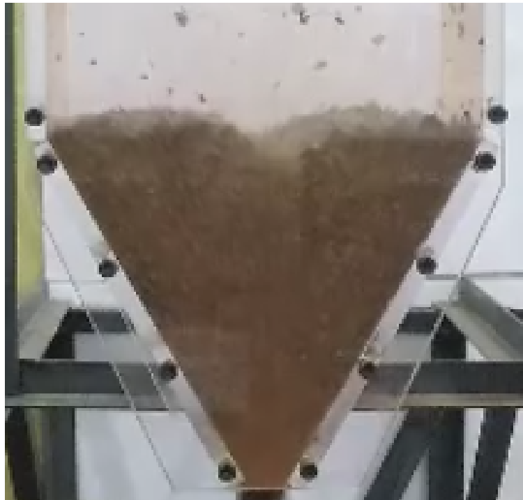
Figure 4.46: Flow profiles comparison, half full silo, moist
