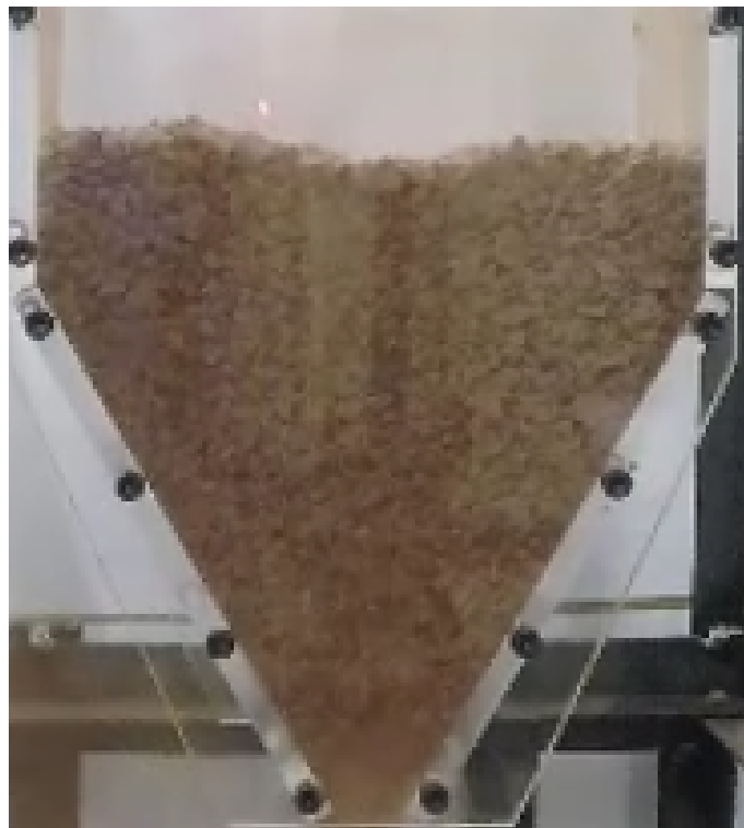
Figure 4.22: Profile of physical silo three quarters full of dry iron ore
