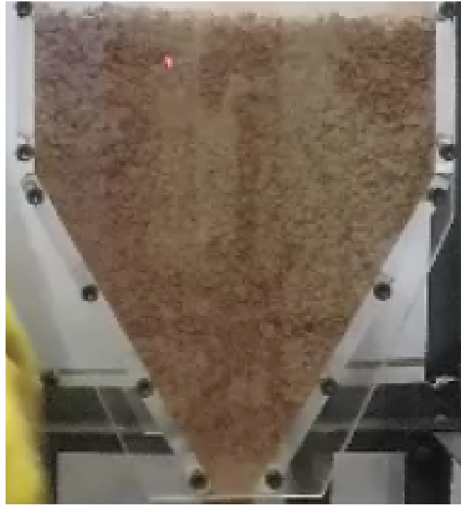
Figure 4.21: Profile of physical silo full of dry iron ore
