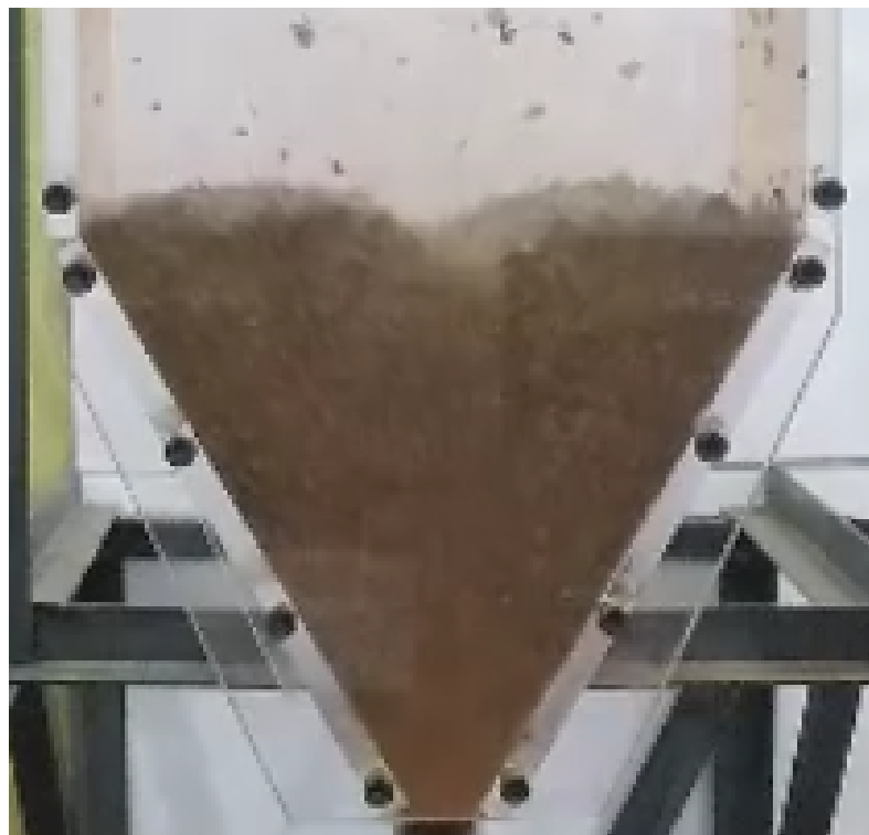
Figure 4.28: Profile of physical silo half full of moist iron ore
