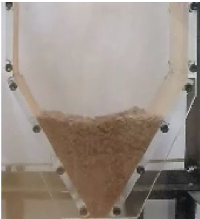
Figure 4.24: Profile of physical silo one quarter full of dry iron ore
