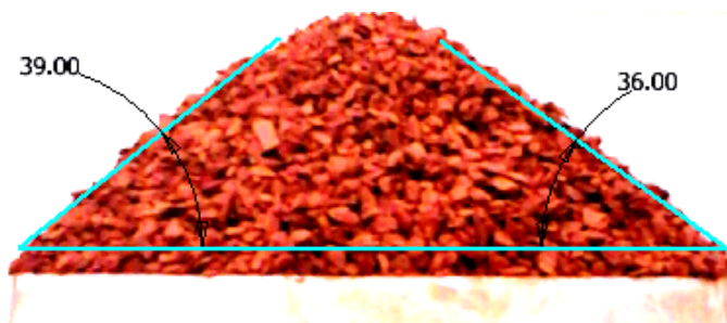
Figure J.4: Full pipe angle of repose, dry, physical test 1 @ 110 mm
