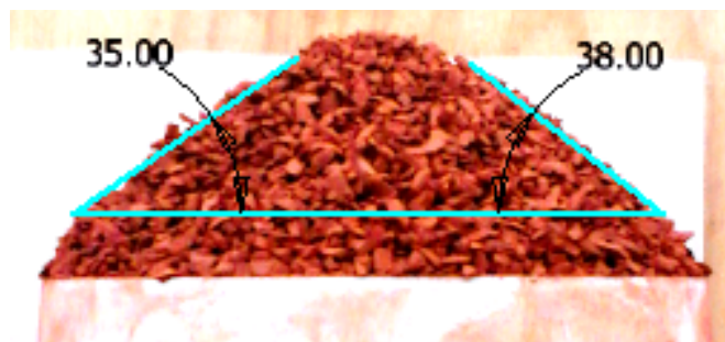
Figure J.6: Full pipe angle of repose, dry, physical test 3 @ 110 mm
