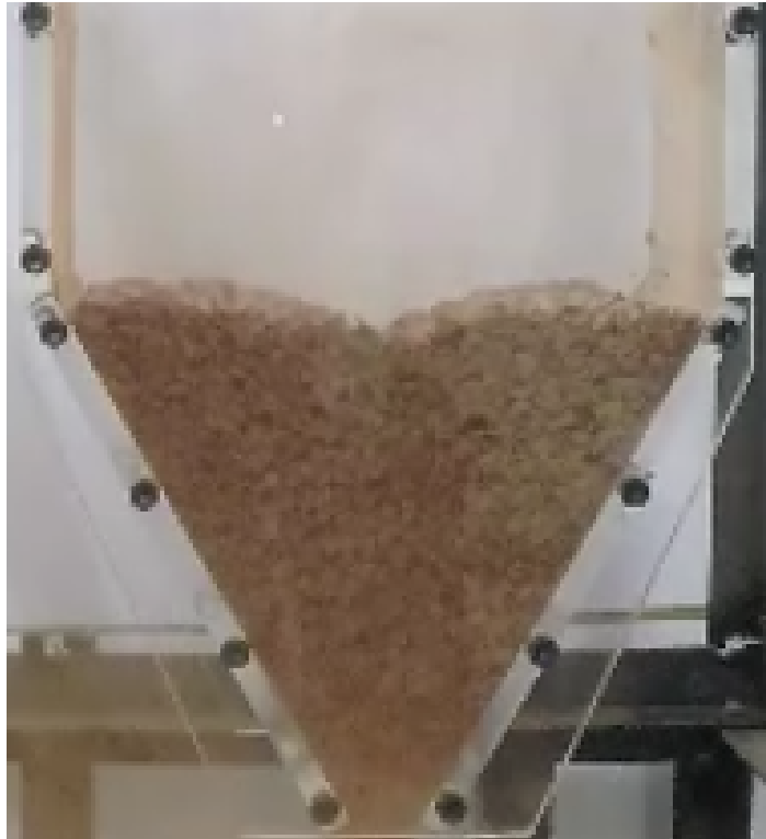
Figure 4.23: Profile of physical silo half full of dry iron ore
