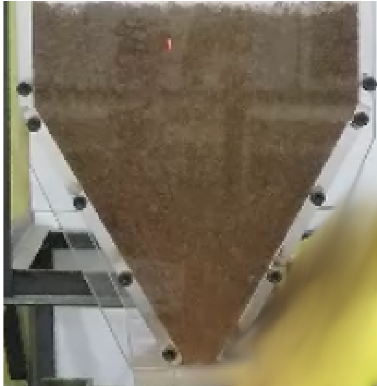
Figure 4.27: Profile of physical silo full of moist iron ore
