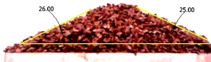
Figure M.1: Split pipe angle of repose, moist, physical test 1
