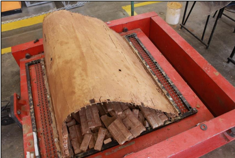
Figure 5.31: Mortar-geogrid composite remained fairly intact after the arch failed
