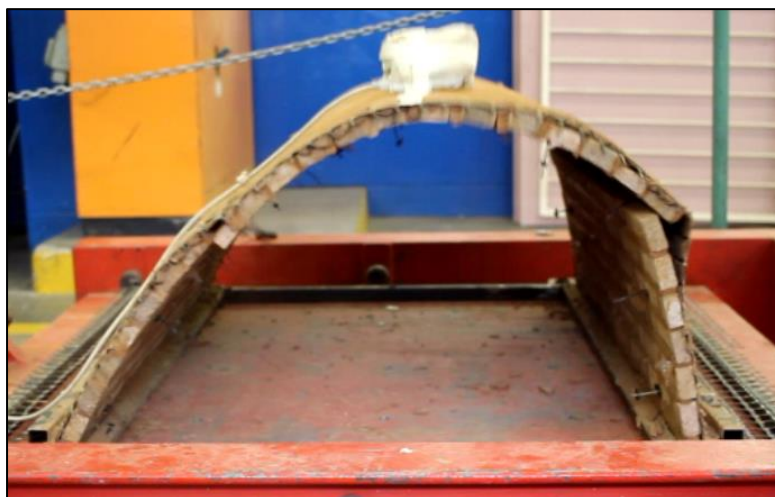
Figure 5.34: Sliding of brick layers is the failure mechanism
