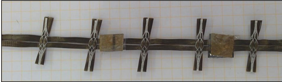
Figure 4.15: Sandpaper attached on either side of the sample at the clamping points
