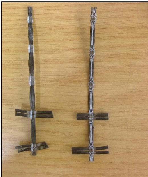
Figure 5.23: Anchors made from basalt fibre geogrid (top and bottom view)
