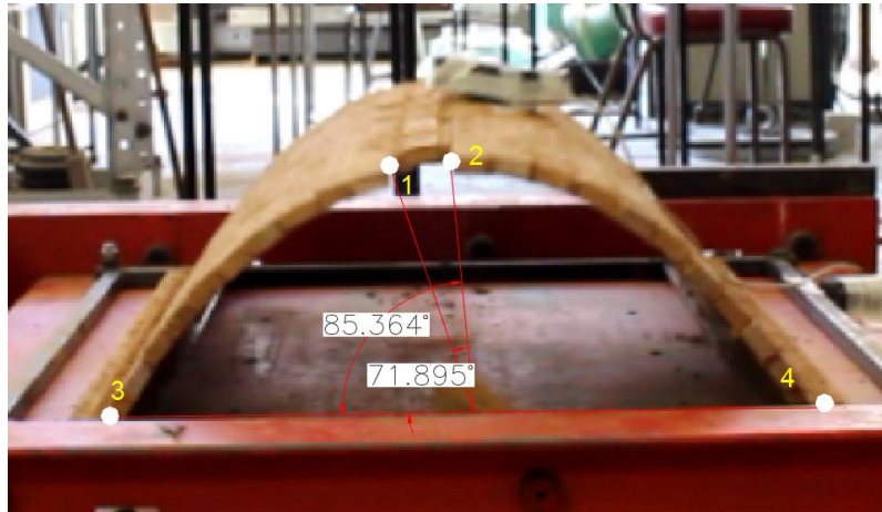
Figure 5.15: Hinge locations 0.8 h/w ratio test (2 Hz)
