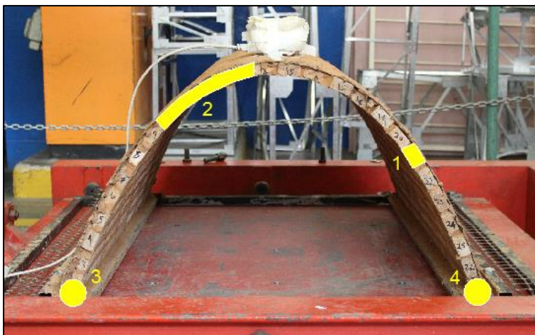
Figure 5.30: Locations of failure points along arch for geogrid only test
