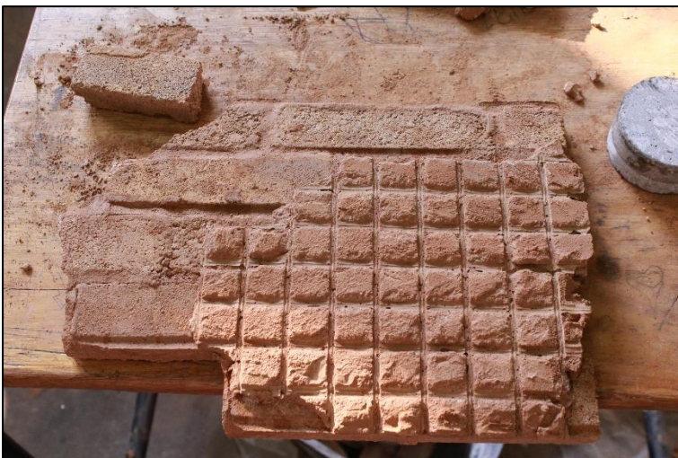
Figure 5.32: Mortar bonded well with the arch
