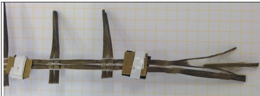
Figure 4.16: Failure only encountered in one of the sub-ribs
