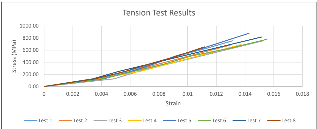
Figure 4.19: Stress v strain graph for basalt fibre geogrid tests
