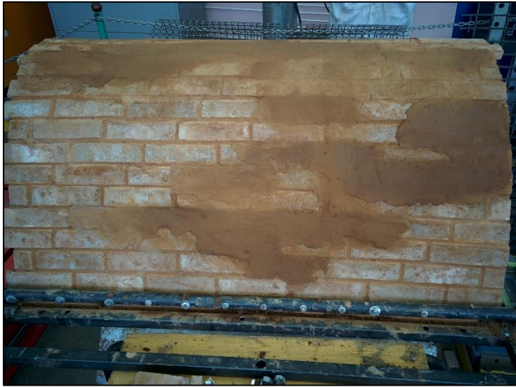
Figure 5.28: Discrepancies in arch depth rectified with mortar
