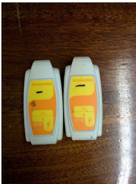
Figure 4.5: Accelerometers connected to the Nova 5000 data logger
