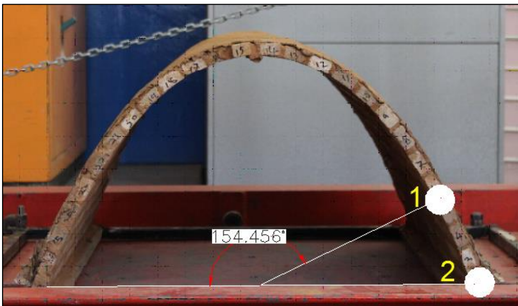
Figure 5.35: Failure points of prestressed arch
