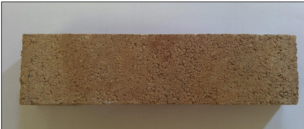
Figure 4.9: A brick cut from an earth tile used in the masonry arches
