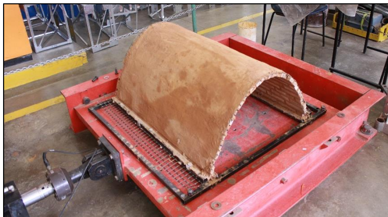
Figure 5.22: Mortar applied over the geogrid
