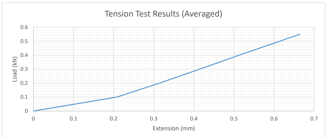
Figure 4.18: Averaged force v extension graph for basalt fibre geogrid tests
