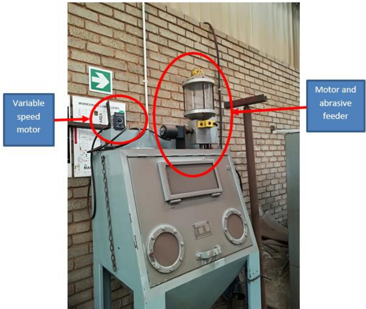
Figure 27: Erosion rig setup
