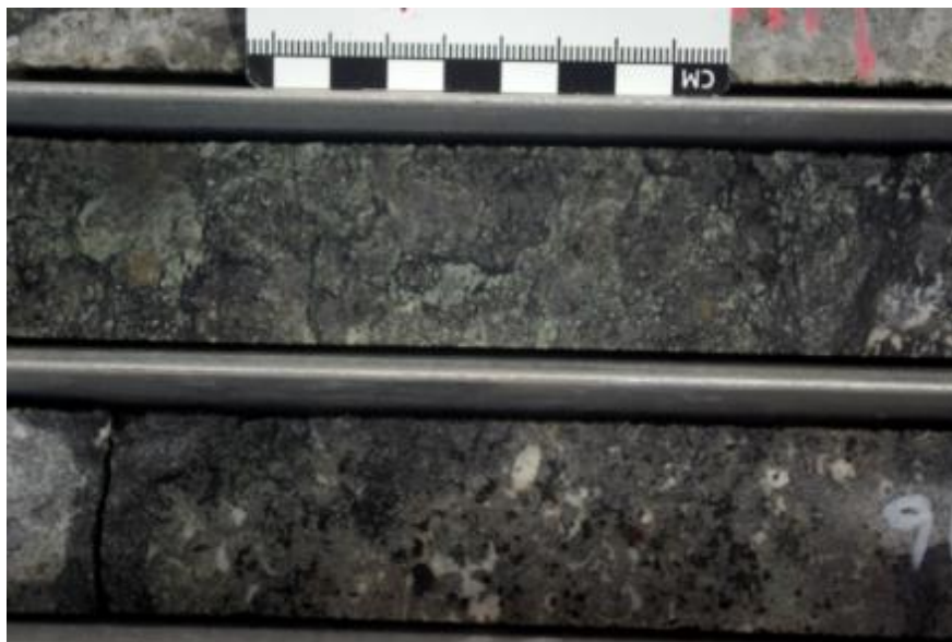
Figure 2.17: Parapyroxenite associated with serpentine in borehole ZF 116 (~1445 m depth). In some cases (bottom) plagioclase is observed with completely serpentinised grains (black).
