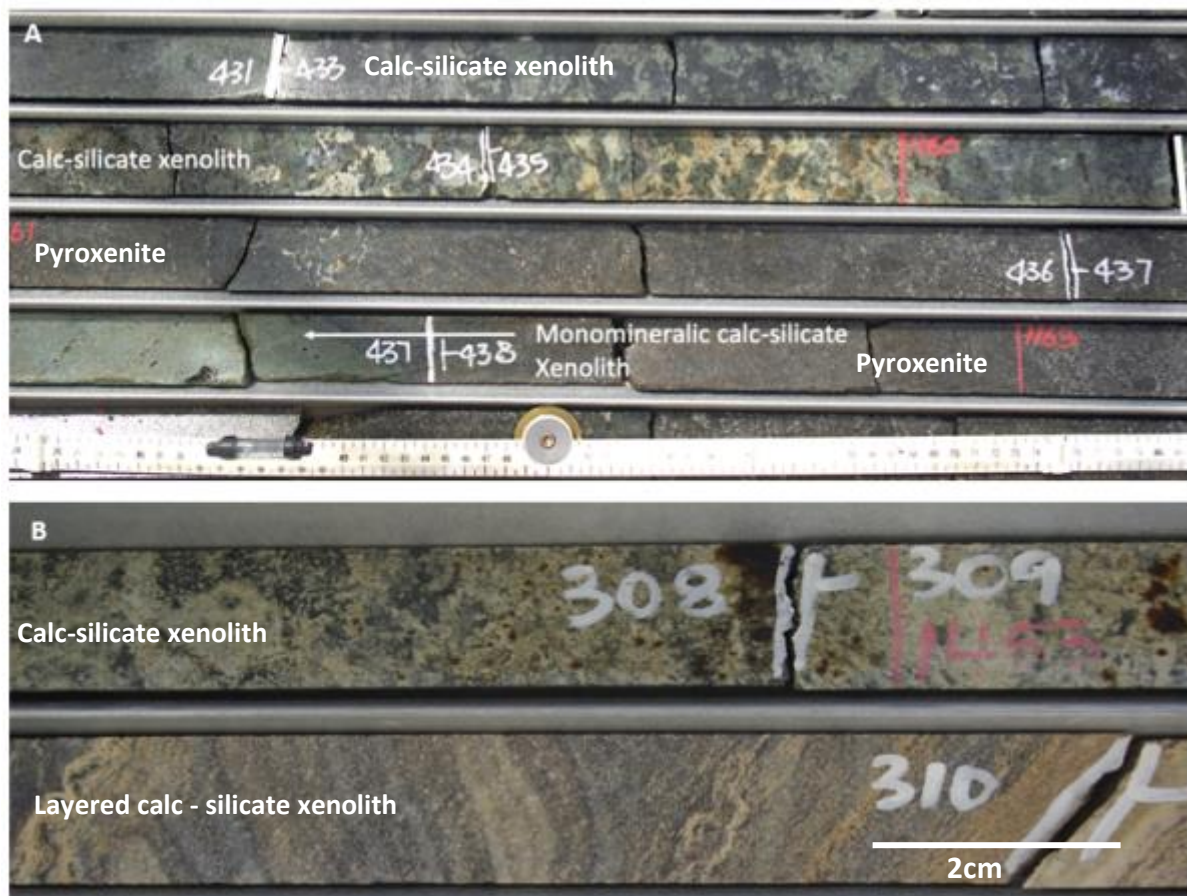
Figure 2.15: Borehole core (A) ZF 109 ED 1 that intersects coarse-grained monticellite, forsterite and clinopyroxene xenolith (top) displaying green, grey and cream to white colours (~1155 m) and medium-grained, green monomineralic (clinopyroxene) xenolith in borehole (~1162 m). (B) Borehole ZF116 showing medium-grained xenolith (top) that comprises clinopyroxene and calcite (~1453 m) and grades into fine-grained layers (bottom) of serpentine, calcite and other Ca-bearing silicates (~1454 m).
