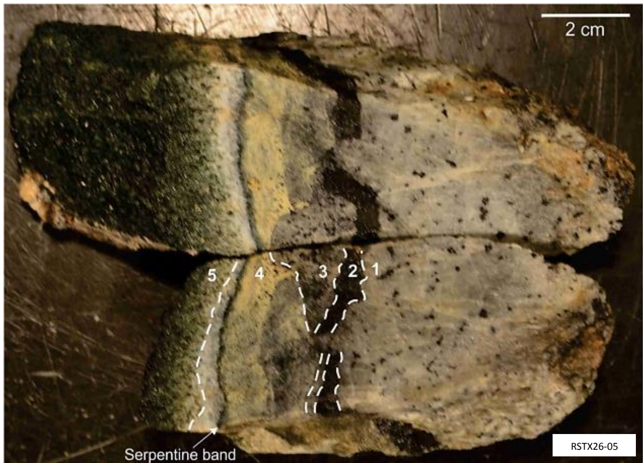
Figure 2.4: Hand sample (RSTX26-05) showing the zonation of minerals immediately adjacent to the xenolith. (1) The forsterite-spinel layer adjacent to the spinel layer (2). This is followed by forsterite-monticellite layer (3), followed by the vesuvianite layer (4), within which a serpentine band occurs, and the clinopyroxene layer (5).
