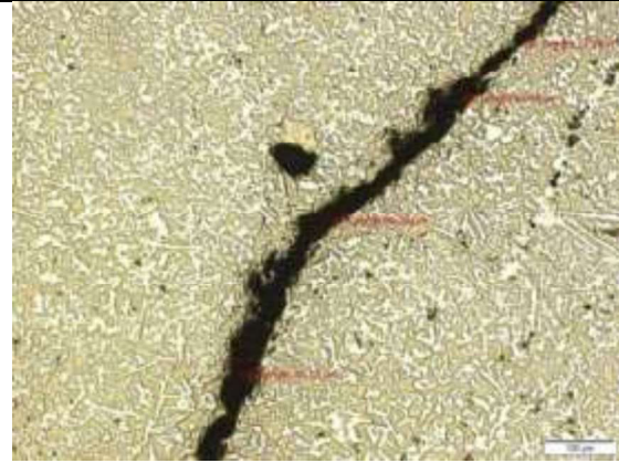
Figure 4.190: Optical micrographs displaying crack lengths of heat treated TiAlMn-1
