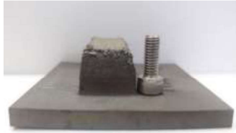
Figure 3.13: Display of height of reprinted TiAlMn-1 (20mm)
