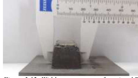
Figure 3.12: Width measurement of reprinted TiAlMn-1 (20mm).
