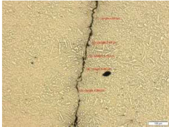
Figure 4.130: Optical micrograph of crack length of as produced Ti-Mn-10.
