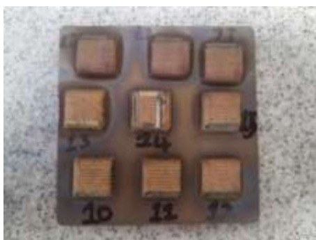
Figure 3.4: Ti-Mn samples printed on Ti-6Al-4V substrate.
