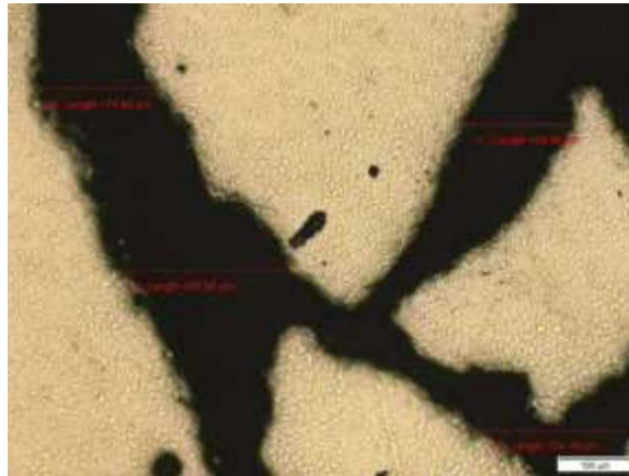
Figure 4.132: TiMn-8 contains largest phase proportion of \text{Mn}_{0.52}\text{Ti}_{0.48}(\text{s}) in Ti-Mn alloys and is the most brittle TiMn alloys and has lowest calculated ductility.
