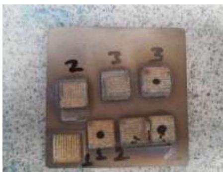
Figure 3.5: TiAlMn sample printed on Ti-6Al-4V substrate
