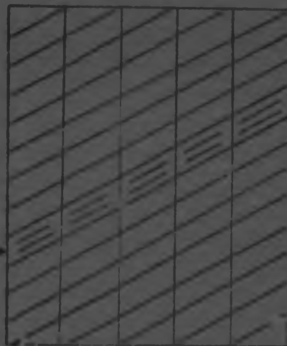
FIG. 3.2A A NON-RECTANGULAR GRID SYSTEM USED TO SIMULATE A VEIN DEPOSIT
