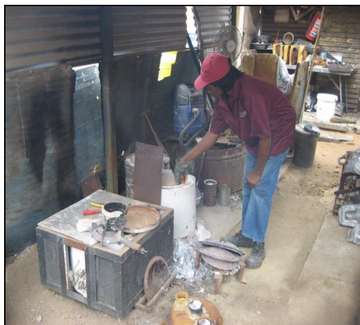
Sikeli MOYO operating the gas fired crucible furnace
