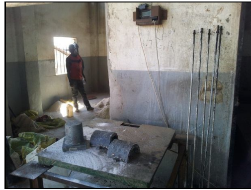
Figure 3.3b: Newly cast permanent mould (Zalco Ltd., April 2014)
