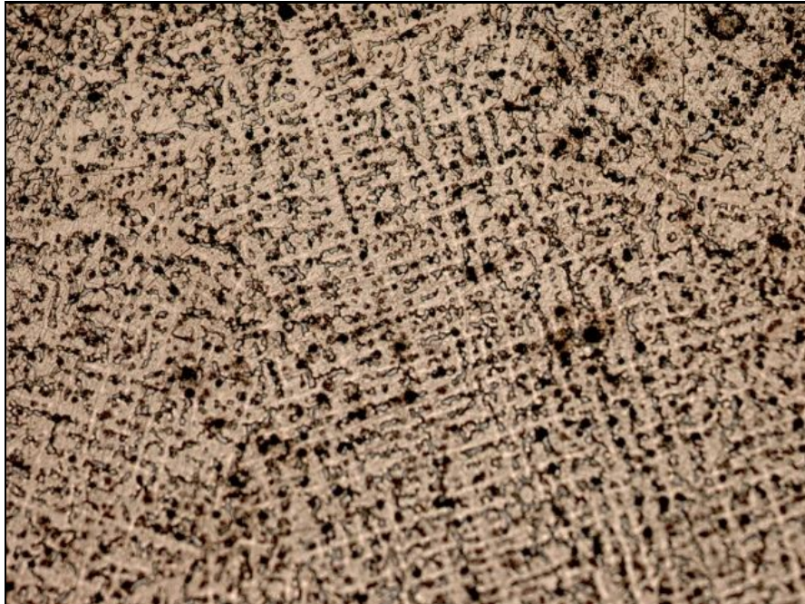
Figure 4.1.5i: Cast sample (Univ. of Joburg WAX, 100X)
