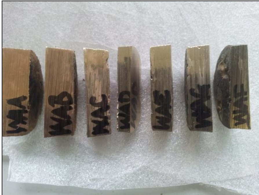
Figure 4.3k: Sections of castings prepared for metallographic and wear testing
