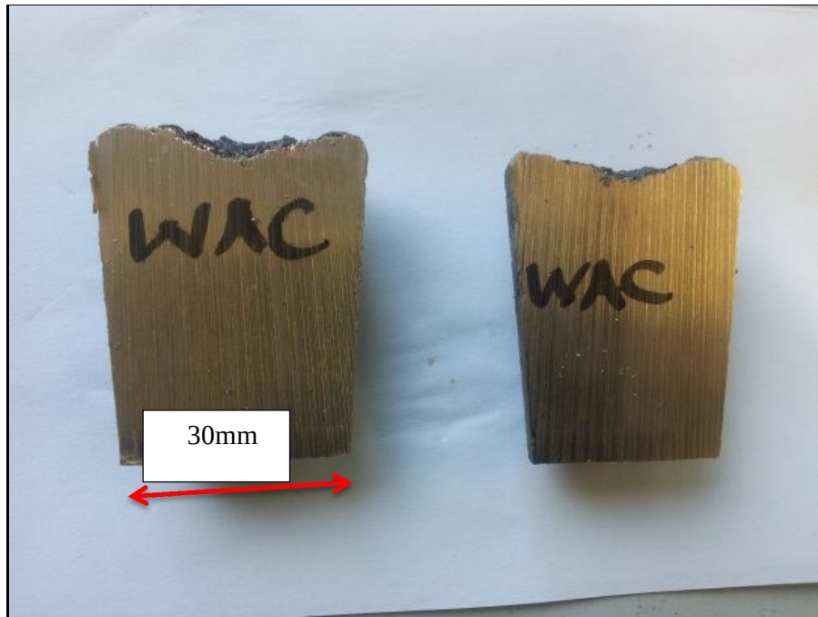
Figure4.3i: Section through casting WAC (dimension of arrow is 30mm)
