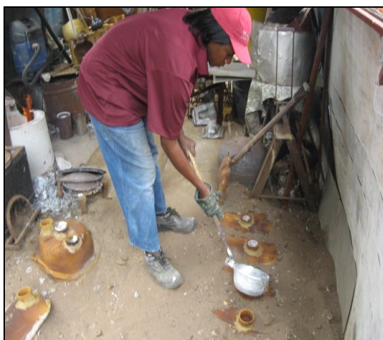
Pouring aluminium metal into various moulds
