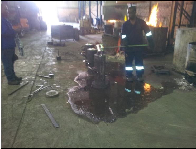
Casting of aluminium ingot bars in permanent moulds at WAM (29 th Aug, 2013)
