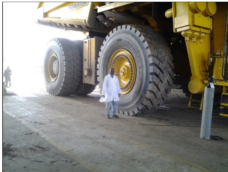
Figure A12: Open pit haulage trucks of payload 200 tonnes use massive bronze cylinders in their hydraulic systems (June 2013)
