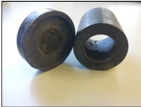
Figure 3.3g: Mould barrel and base
