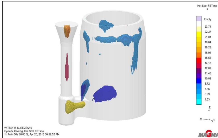
Figure 4.3c: Likely hot spot locations in terms of portions of extended solidification times (Simulation by Ametex, April 2015)
