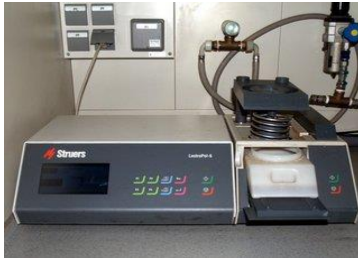
Figure 3.4: Struers LectorPol-5 electropolishing machine.
