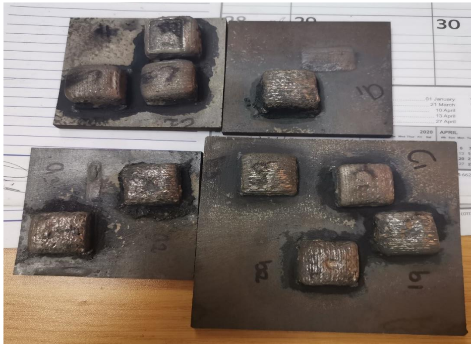
Figure 3.2: DED samples produced using the KUKA robot.
