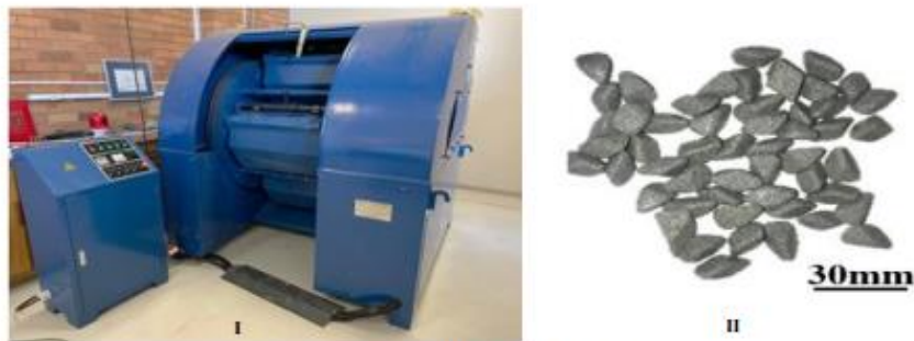
Figure 2. CB320-CBF Machine (I) and ceramic media (II)
