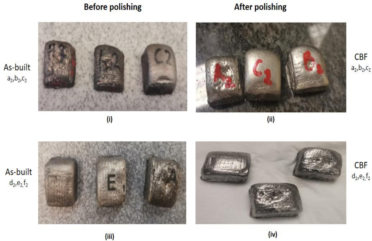
Figure 4.23: DED untreated as-built samples (i) (iii) and CBF treated samples (ii) (iv).
