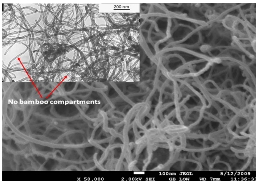
Fig. 9.1 (b). A SEM and TEM image (inset) of MWCNTs synthesized using a mixture of 10% FcH in toluene.
