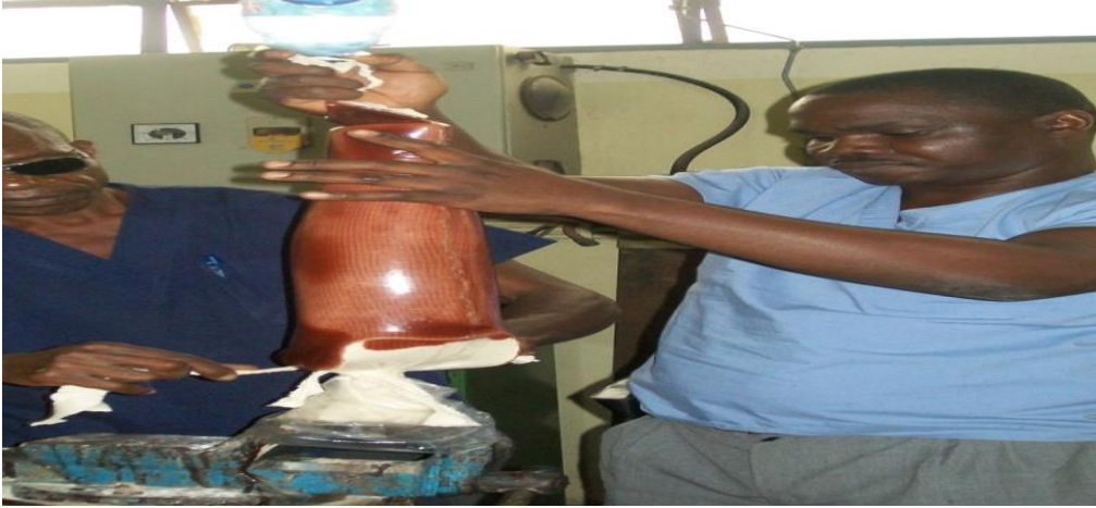
Photo 1. Moulding process with plaster made from acrylic resin.
