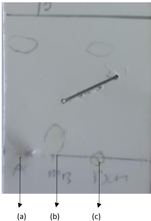
Figure A15. TLC analysis for reductive amination of 58 (30% EtOAc/hexane). (a) Acetophenone standard starting material. (b) MBA standard product. (c) Reaction involving Prozomix-TA038 at 100 mM of acetophenone
