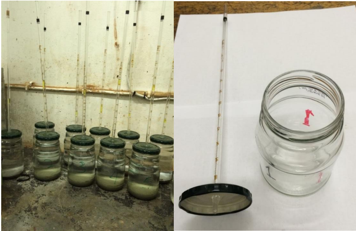
Figure 4.13: Chemical shrinkage measurement apparatus and experimental setup
