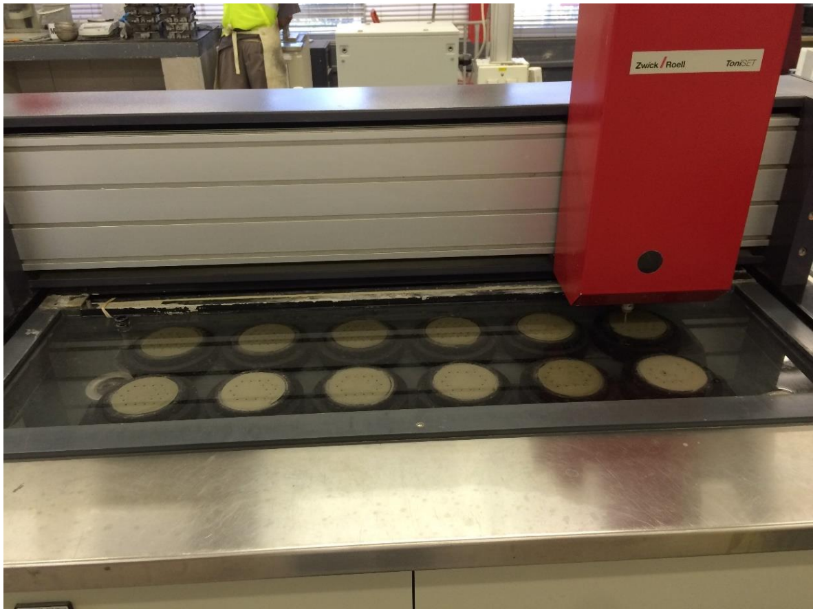
Figure 4.2: An automatic vicat apparatus used in measurement of both initial and final setting times
