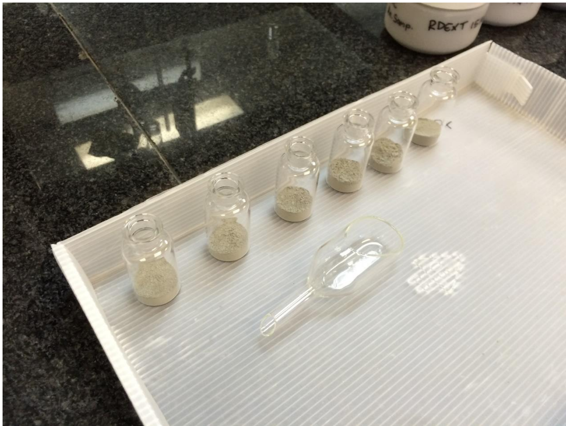
Figure 4.12: Samples placed in ampules ready to be covered and loaded in the isothermal calorimeter for equilibration before water is added and mixing done inside the testing equipment.
