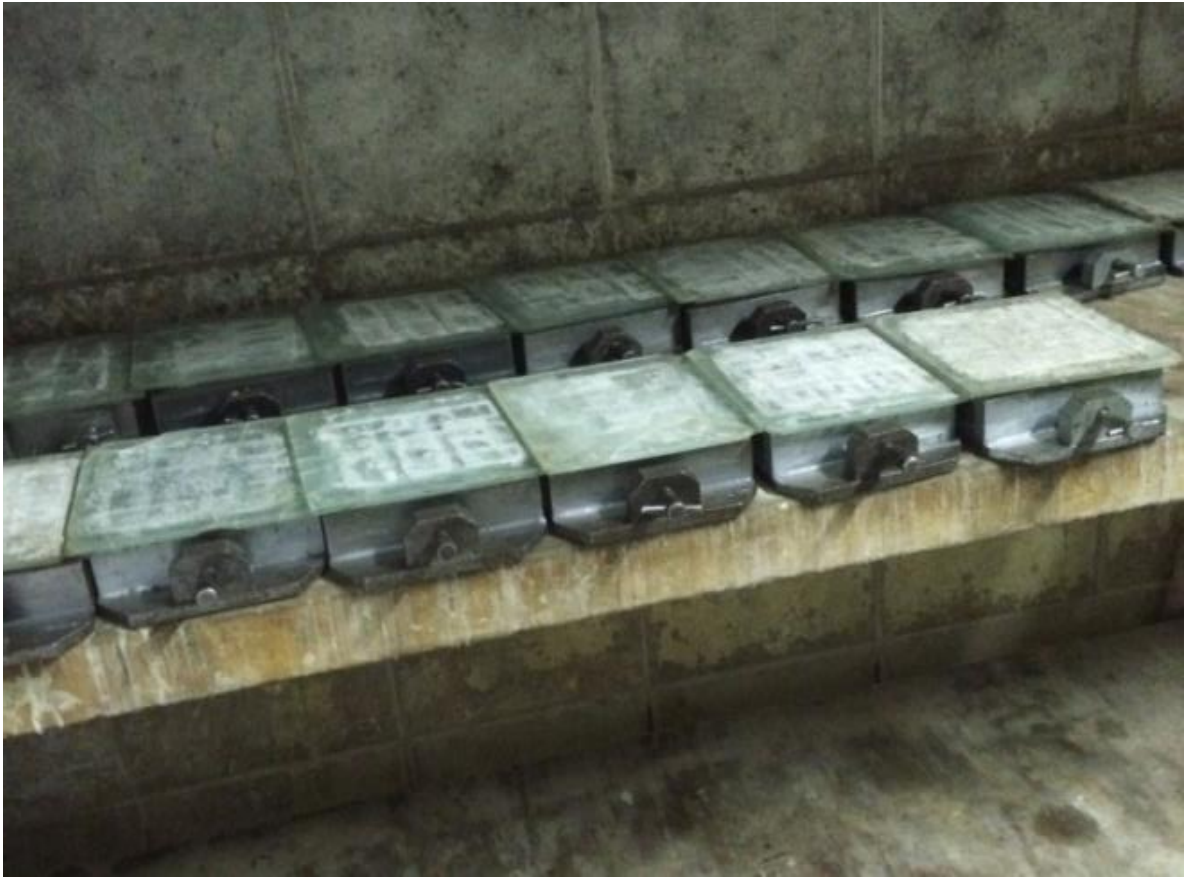
Figure 4.4: Mortar prism samples placed in a curing room and covered with glass for 24 hrs before demoulding.
