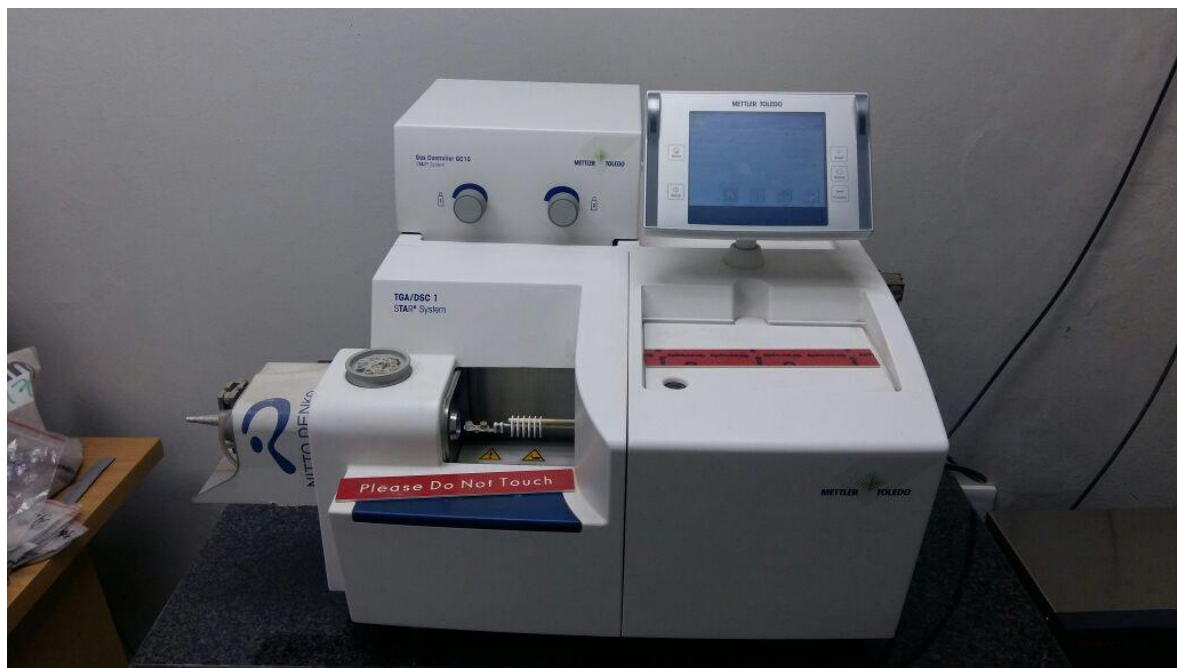
Figure 3.9: Thermogravimetric analysis (TGA) instrument used in characterisation of volatile compounds in kamafugites and carbonatites
