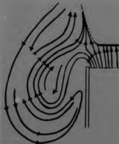
Fig 2.4 Particle track photograph of a flat flame with sketch of direction of observed flow (LW 59)
