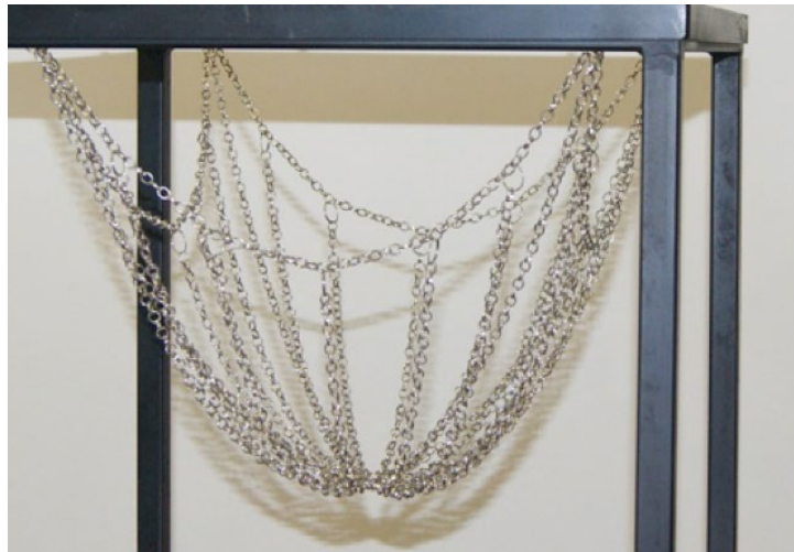
Figure 4.4 – Hanging chain model supported in the corners
