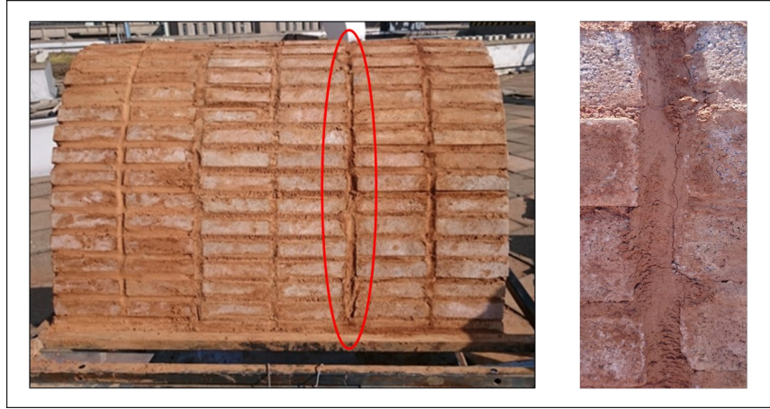
Figure 7.15 – Vertical crack in a catenary vault model
