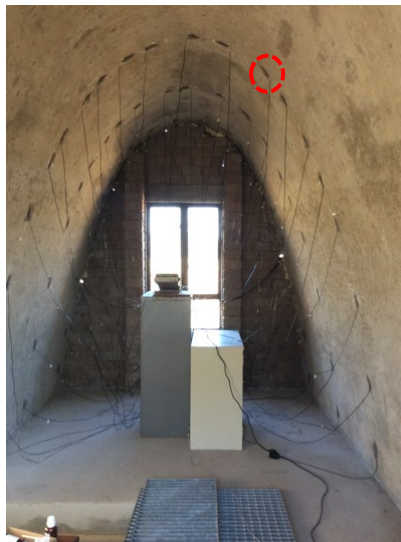
Figure 6.14 – Thermocouples attached to the internal surface of the south-facing shell
