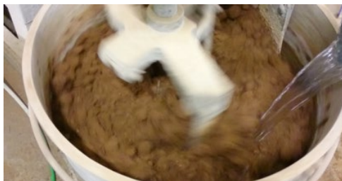
(c) Mixing the cement, soil and water
