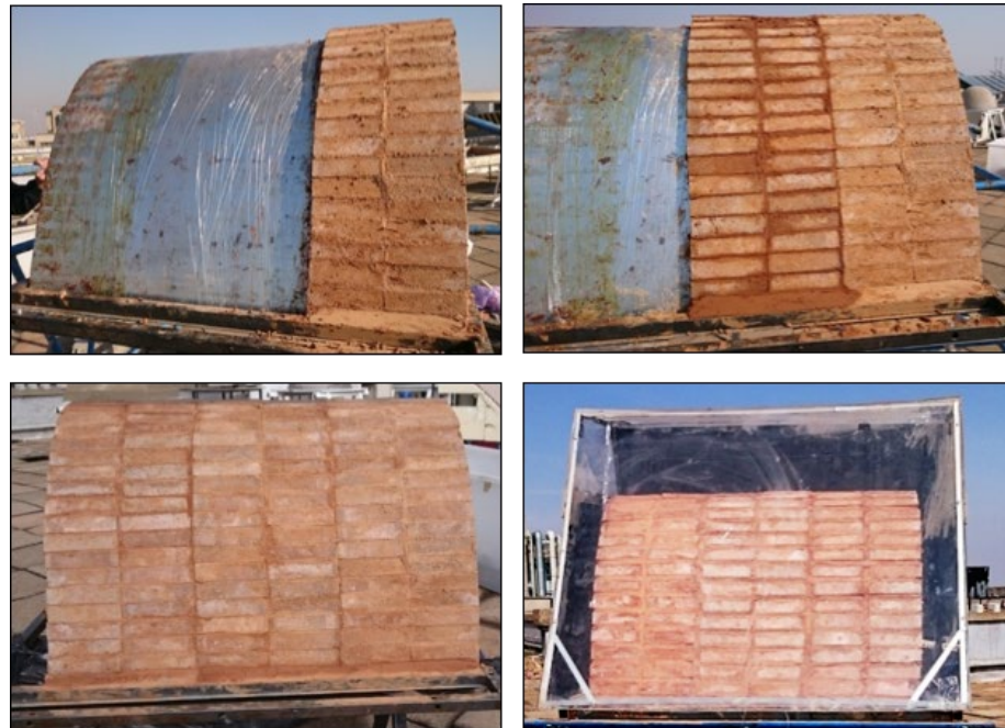
Figure 7.14 – Construction sequence of a vault model
