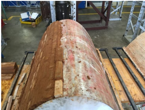
(a) Small scale catenary vault construction (b) Shrinkage prevented by rigid formwork
