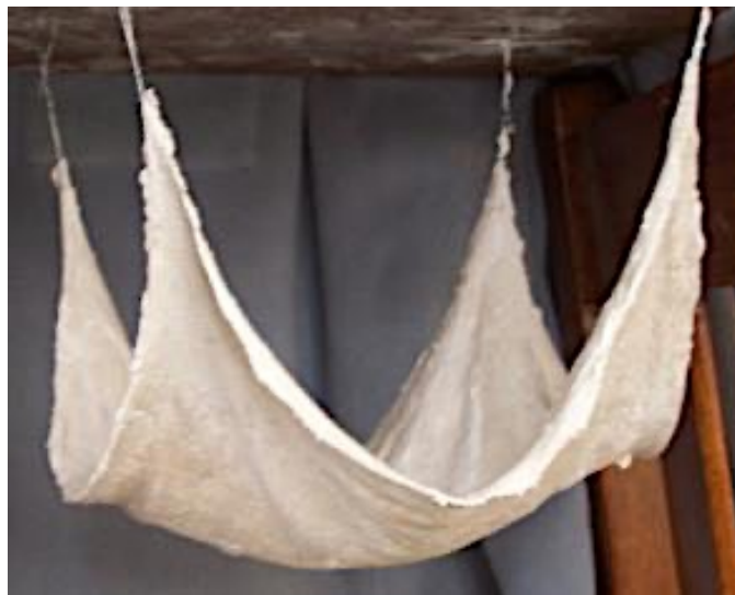
Figure 4.3 – Cloth model supported in the corners (Image courtesy of Mitchell Gohnert)
