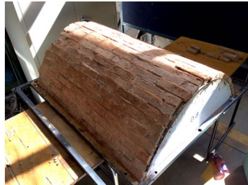
(a) Small scale catenary vault construction (b) Shrinkage prevented by rigid formwork
