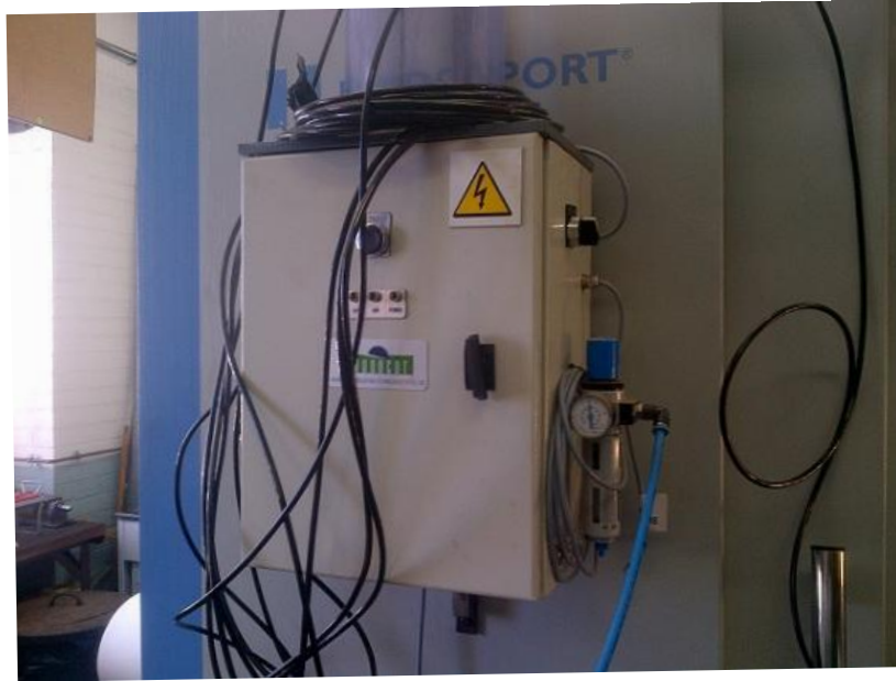
Figure 3.15: Product MQL system mounted onto the Bridgeport GX100 CNC milling machine
