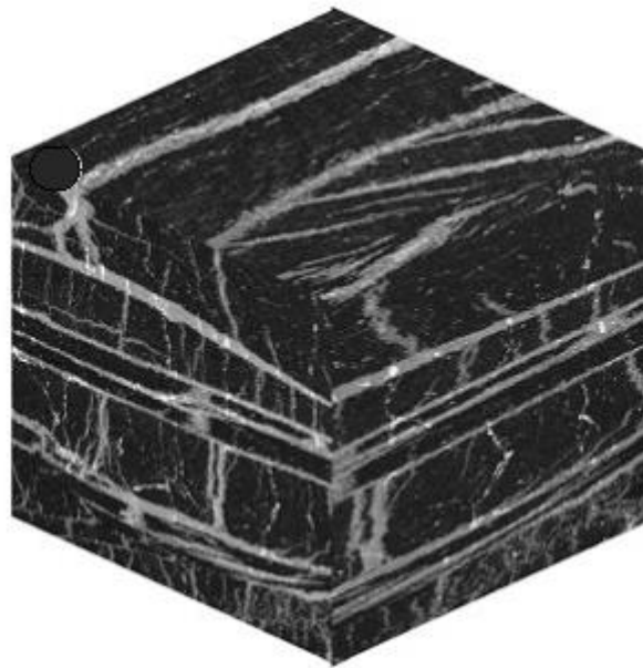
Figure 12: The typical microstructure of a C f /SiC composites (Jiang et al. , 2008).
