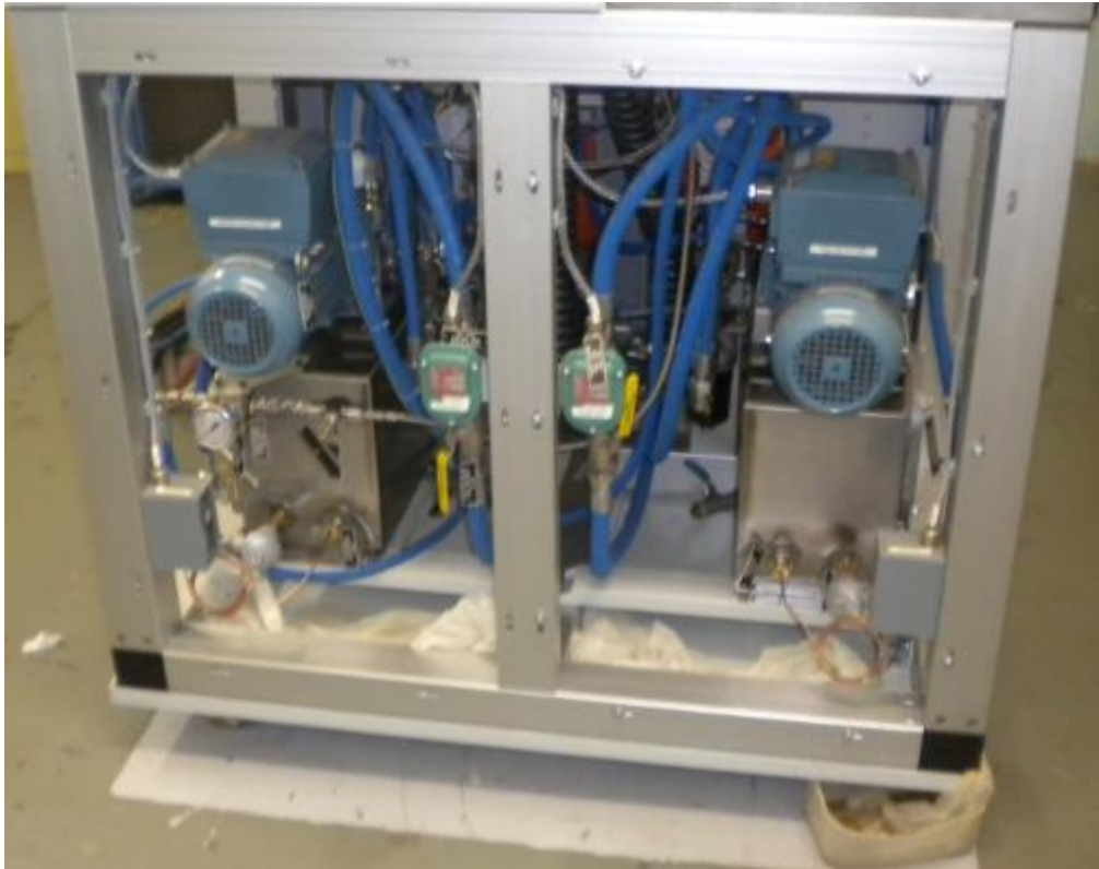
Figure 20: Cooling fluid and test fluid tanks
