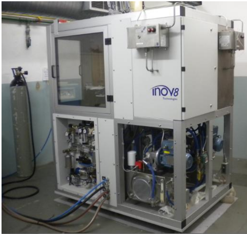
Figure 17: Spray pattern analysis and flow measurement test stand
