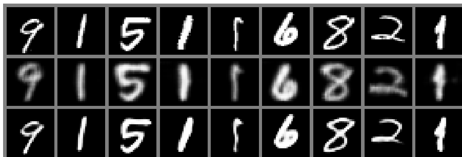
Figure 7.1: Example image output for our model on MNIST→USPS. Row 1 is the original image from MNIST, row 2 is the fake USPS image generated from the GAN and the final row is the reconstructed MNIST image.
