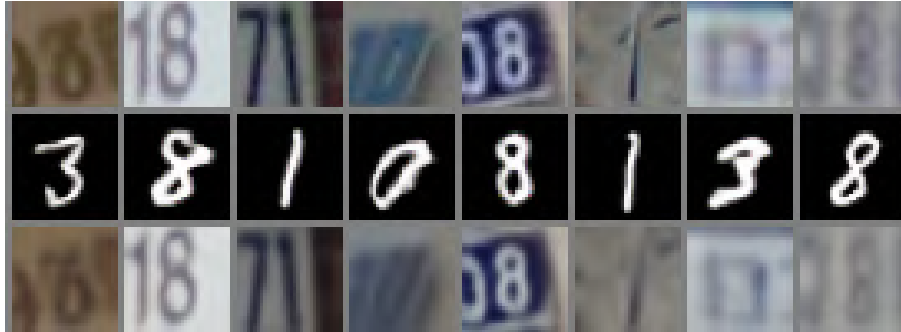
Figure 7.3: Example image output for our model on SVHN \rightarrow MNIST. Row 1 is the original image from SVHN, row 2 is the fake MNIST image generated from the GAN and the final row is the reconstructed SVHN image.
