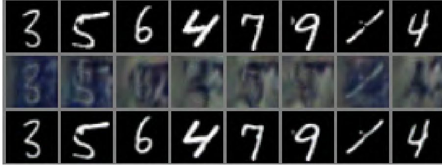
Figure 7.4: Example image output for our model on MNIST→SVHN. The first row is the original image from MNIST, the second row is the fake SVHN image generated from the GAN and the final row is the reconstructed MNIST image.
