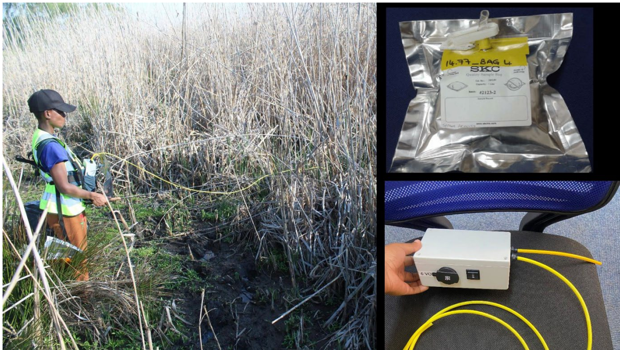
Figure 11: Sampling equipment (flexfoil bag, fishing rod, and 6V battery operated pump).
