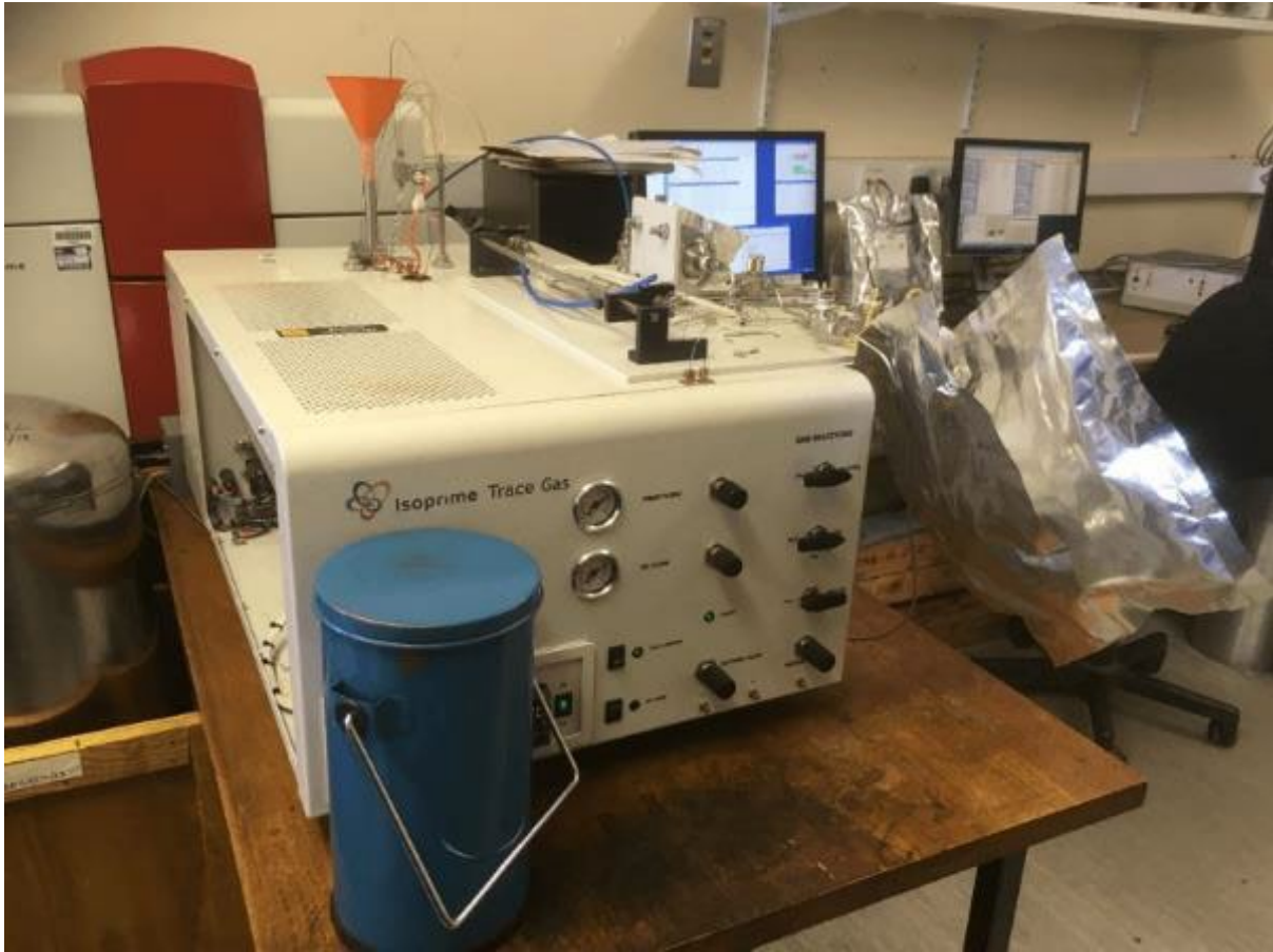
Figure 18: Image showing the CH 4 analyser during sample analysis. Reproduced from Fisher et al. (2006).
