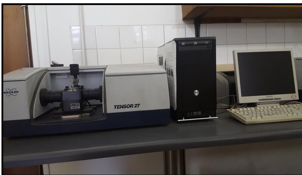
Figure 3.10 Bruker Tensor 27 FTIR analyser.
