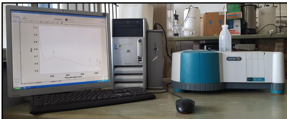
Figure 3.13 Varian UV-vis spectrophotometer.
