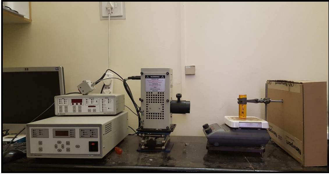
Figure 3.14 Newport Illuminator Solar Simulator Oriel Instruments WX00048.
