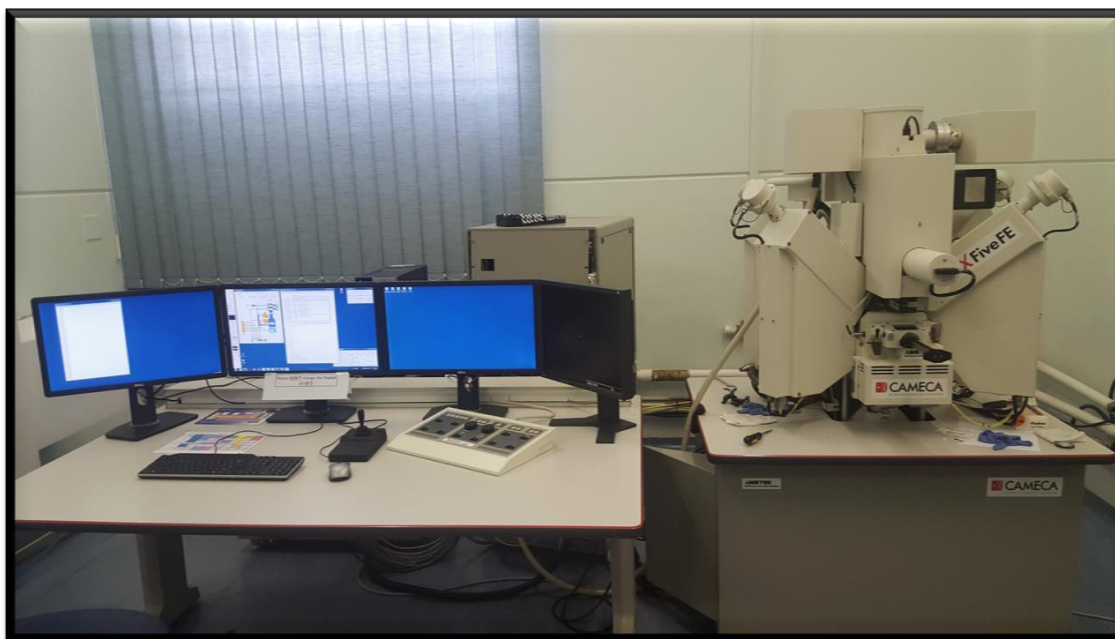
Figure 3.4: The electron probe micro-analysis assembly.
