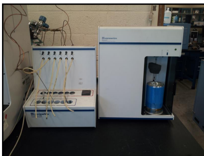
Figure 3.9 Micromeritics RS232 Brunauer -Emmett-Teller (BET) surface area analyser.
