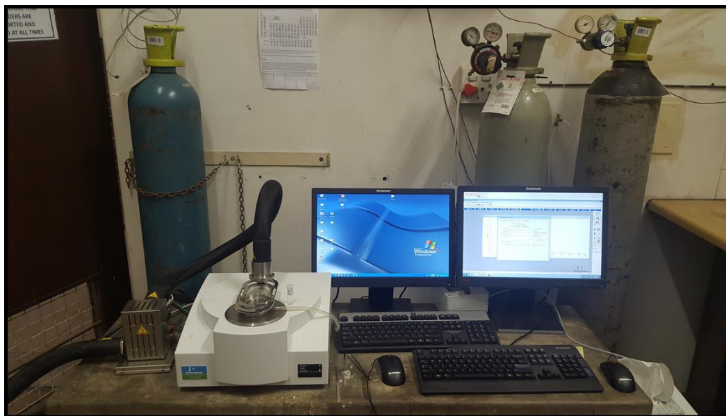
Figure 3.12 TGA – MS Simultaneous Thermal analyser.
