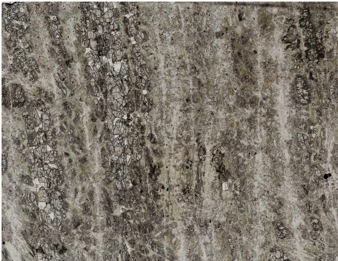
Figure 4. 5: Hybrid rock from UMT335 at 1720 that contains orthopyroxene grains orientated with the layering of the original dolomite protolith.
