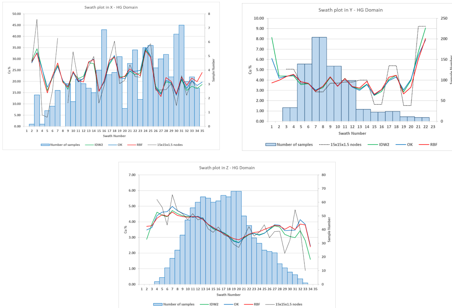
Figure 5.9: HG domain % Cu grade swath plots of the averages of simulated samples, IDW2, OK and RBF block estimates in the X, Y, and Z directions
