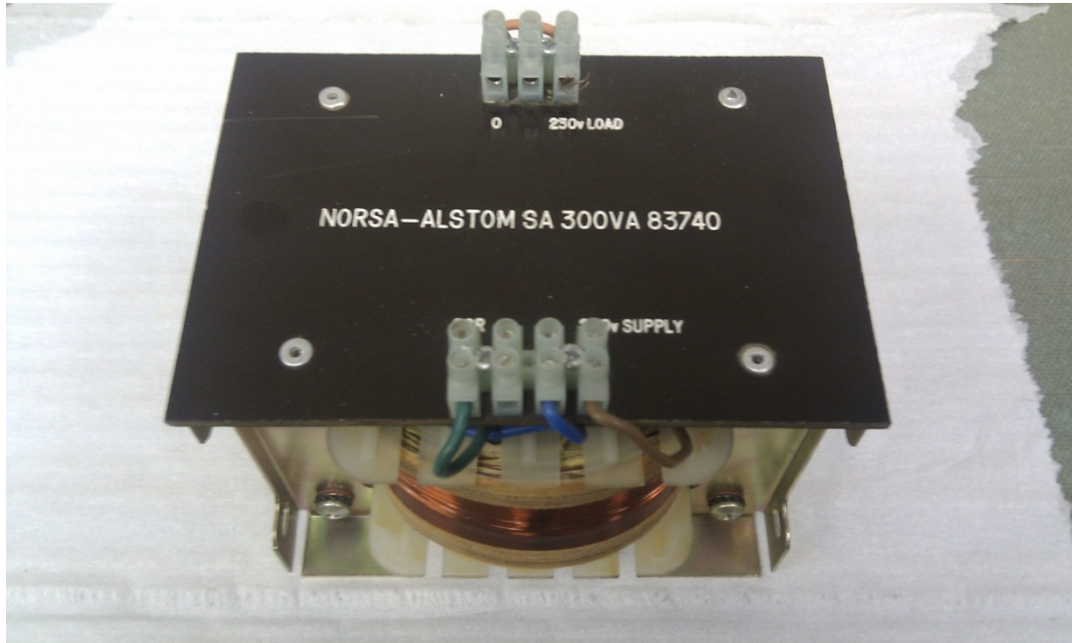
Figure 4: Power transformer under test
