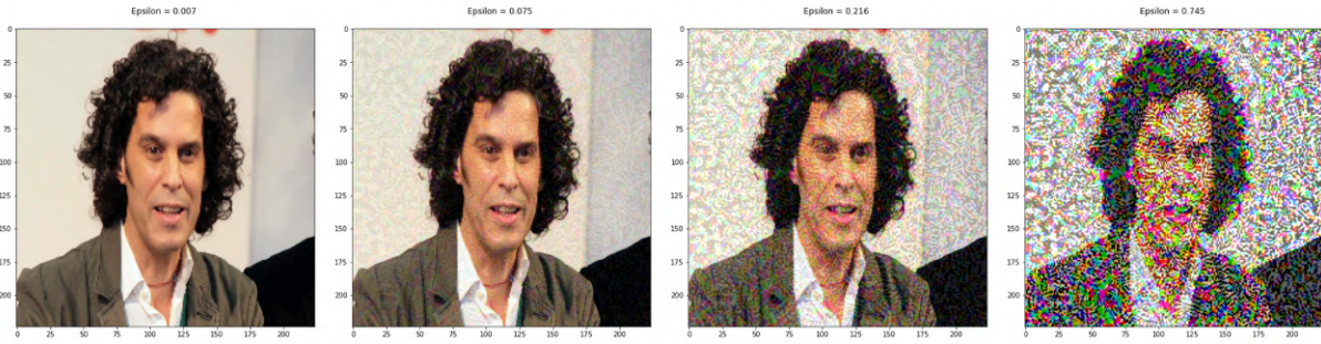
Figure 5.3: One sample of FGSM adversarial attacks created per epsilon. The epsilon values appear as floats because matplotlib turns fractions in the titles to floats
