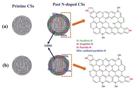
Fig. 6 Possible mechanism showing the role of carrier gas on the N-configuration of the CSs synthesized in the presence of (a) H<sub>2</sub> and (b) Ar, respectively.
