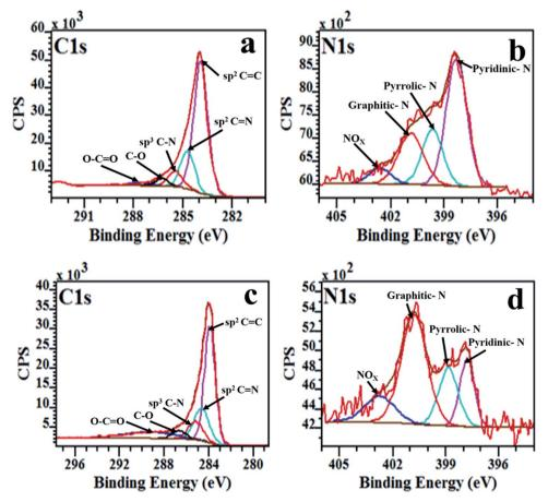
Fig. 4 The XPS spectra of deconvoluted C 1s and N 1s peaks of N-doped CSs; (a and b) NCSs-H<sub>2</sub> and (c and d) NCSs-Ar, respectively.
