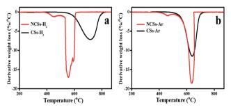
Fig. 3 The TGA derivative weight profiles of the pristine and N-doped CSs; (a) synthesized in H<sub>2</sub> and (b) synthesized in Ar, respectively.
